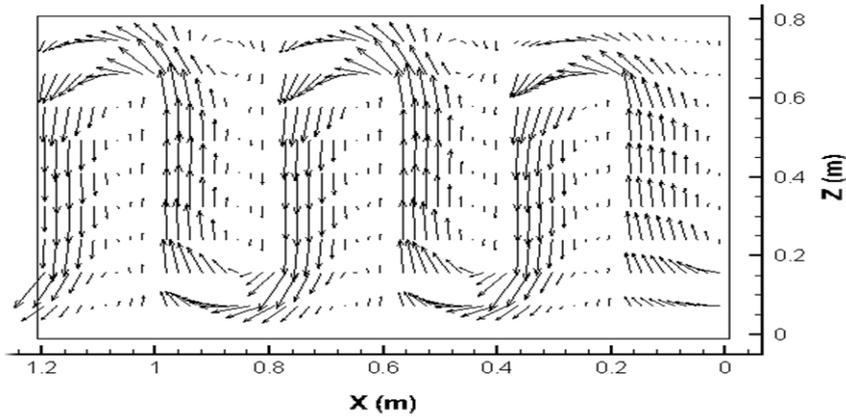
Fig. 10 Velocity vectors of airflow with mass flow rates of 0.05kg/s and duct height of 3.75 cm.
