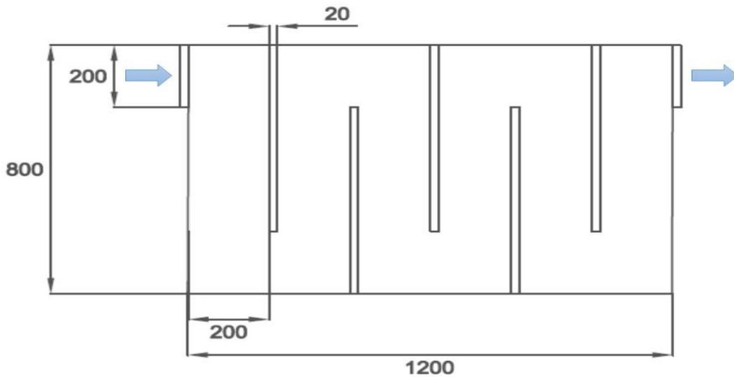
Fig. 1 Upper view of collector with dimensions for numerical and experimental models and directions of flowing air at inlet and outlet
