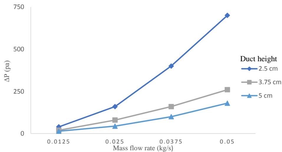
Fig. 7 Numerical Variation of air pressure difference across the duct with mass flow rates for different values of duct height
