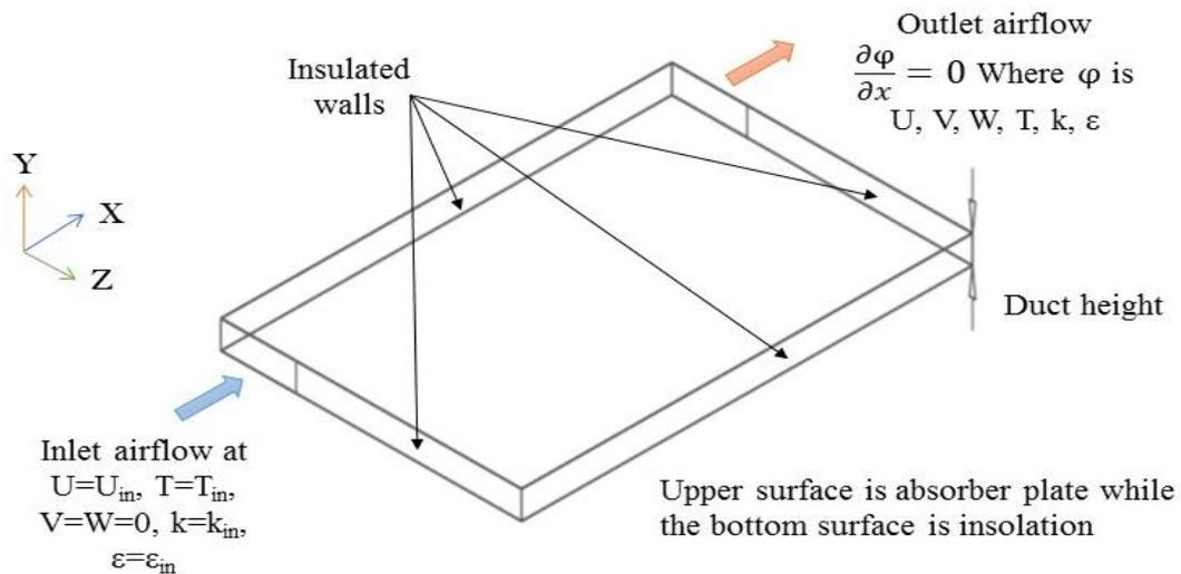
Fig. 2 Schematic diagram of numerical model with boundary conditions
