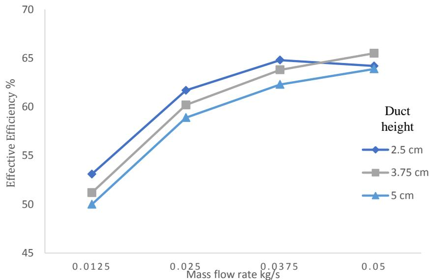
Fig. 9 Variation of effective efficiency of solar air heater with mass flow rates for different values of duct height
