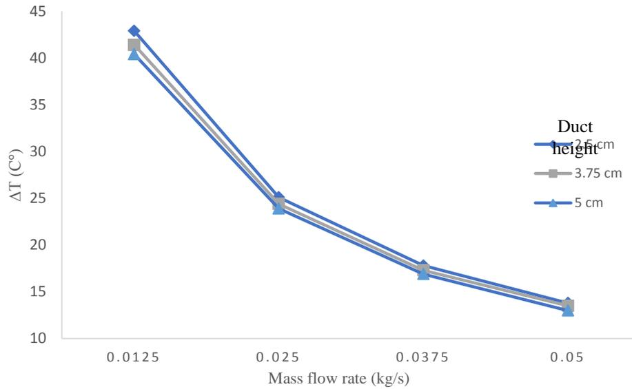
Fig. 6 Numerical Variation of air temperature difference across the duct with mass flow rates for different values of duct height
