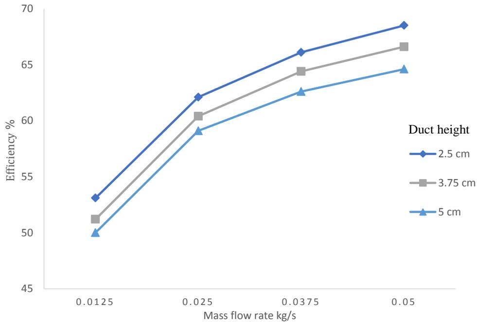
Fig. 8 Variation of thermal efficiency of solar air heater with mass flow rates for different values of duct height
