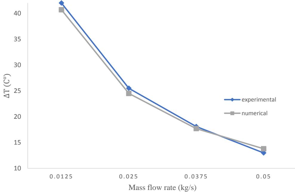
Fig. 5 Comparison between experimental and numerical variation of air temperature difference across the duct with mass flow rate.
