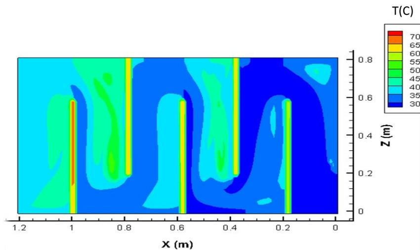
Fig. 11 Temperature contour (x z plane) at  $y = 2.7$  cm with mass flow rate of 0.05 kg/s and duct height of 3.75 cm.
