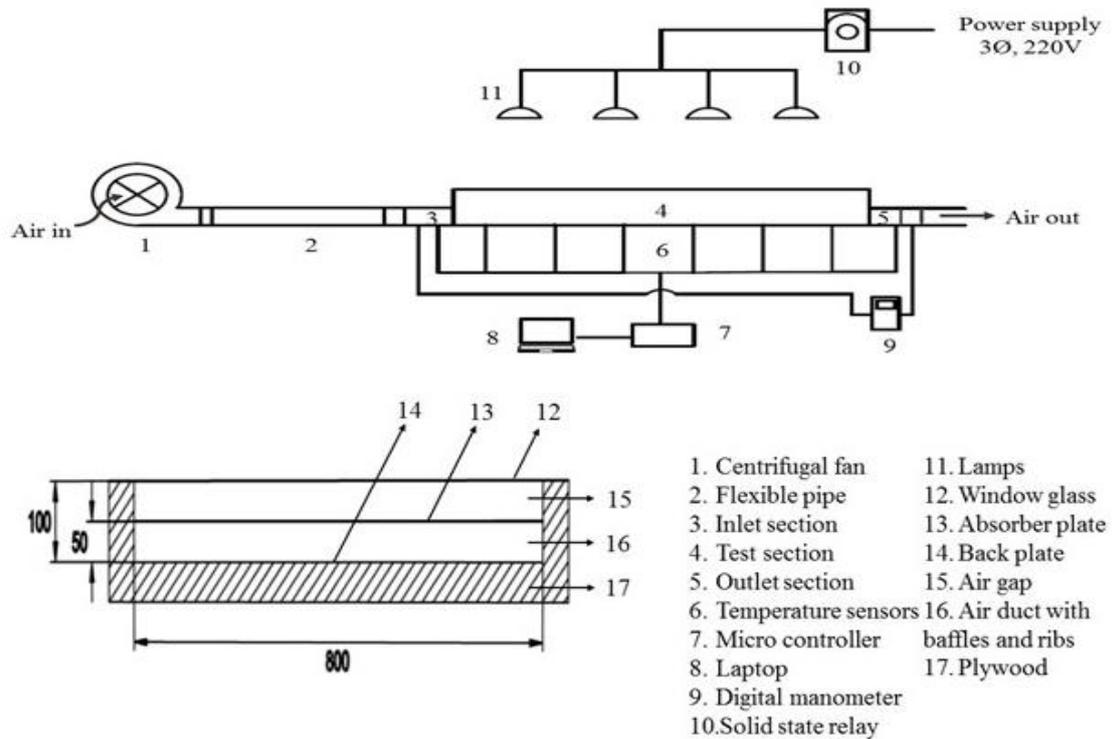
Fig. 3 Schematic drawing of the overall experimental system and cross section of the collector
