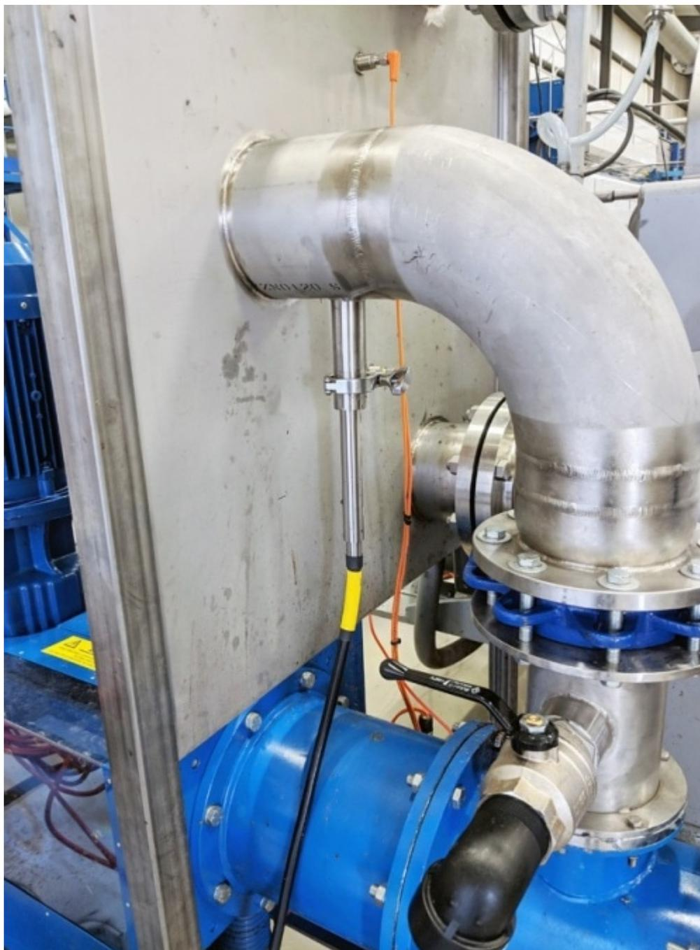
The QuasIR™ 4000 is can be used for both at-line and on-line measurements, being able to analyze paste and pomaces in reflection mode, and oils in transmission mode.
