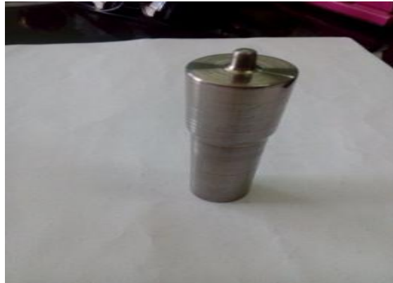
Figure 3 FSW horn tool geometry
