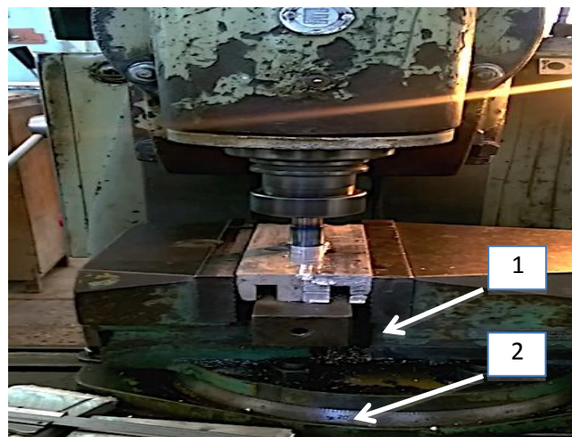
Fig 2. FSW machine, (1) machine vice, (2) supporting plate
