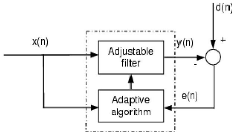
Figure (1) Block Diagram of General Adaptive Filter
