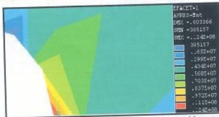
Fig. (6) equivalent stress around crack tip zone of specimen with central circular crack length (25mm)
