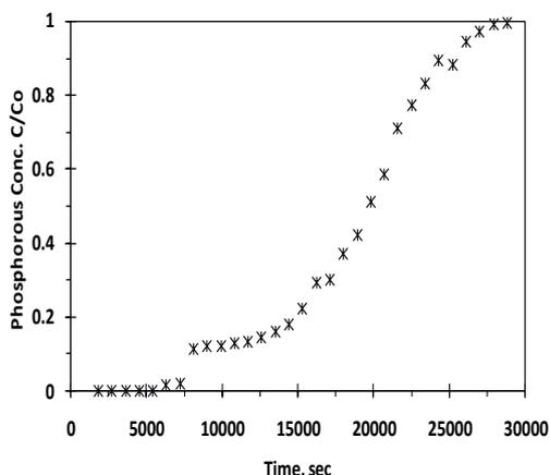
**Fig. 4, Phosphorus ratio (C/Co) concentration with time**
