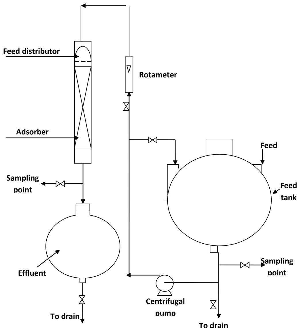
**Fig. 1, Schematic representation of experimental equipment**
