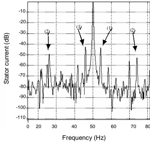
Fig. 10 Stator current power spectra around 50Hz.
