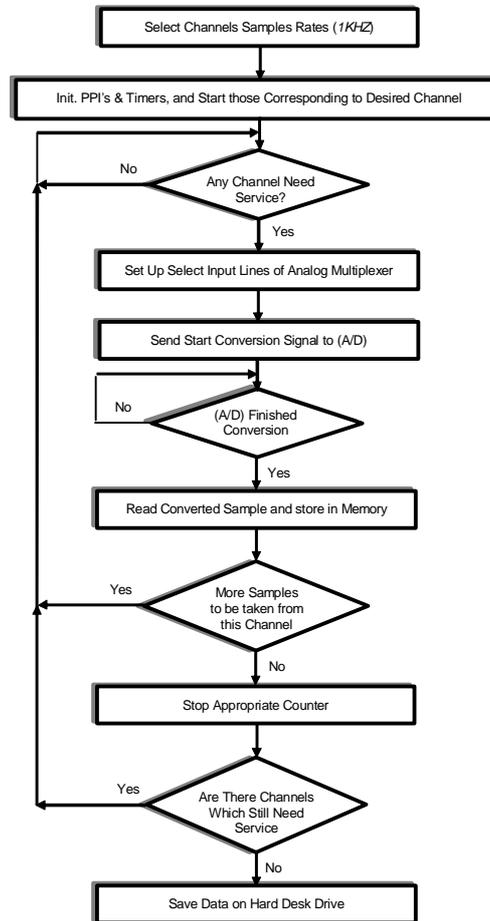
Fig.4 Flow chart of data acquisition software programs.
