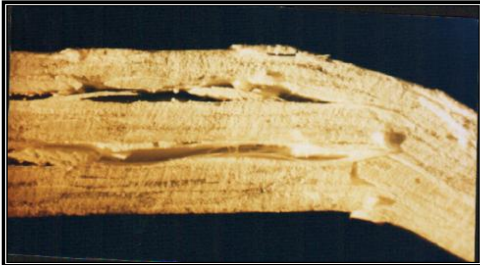
Fig (8.b): Tensile side of the fracture surface of the sample (Ep+ random) 7 layers
