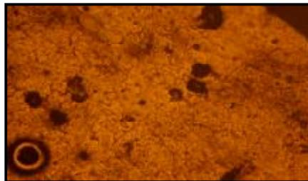
Figure (2) EM pictures of sintered HA powder compact at different Sintering temperatures and at a magnification of (X63) .
