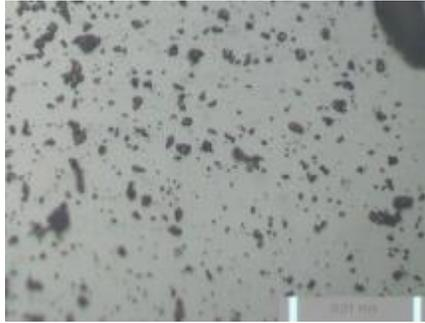
Figure (1) shows the particle shape of fabricated HA
