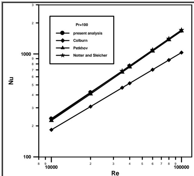
Figure (8) Comparison between Nu Obtained from Present Analysis with Other Works at Pr=100.
