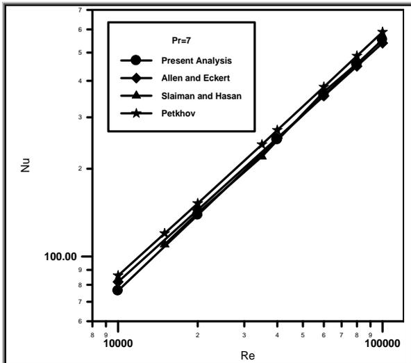
Figure (7) Comparison between Nu Obtained from Present Analysis with Other Works at Pr=7.
