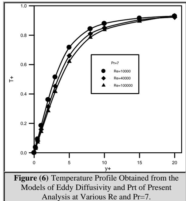
Figure (6) Temperature Profile Obtained from the Models of Eddy Diffusivity and  $\text{Pr}_t$  of Present Analysis at Various  $\text{Re}$  and  $\text{Pr}=7$ .
