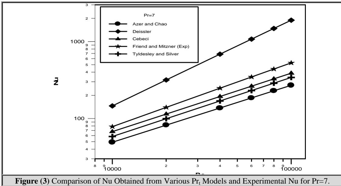
Figure (3) Comparison of Nu Obtained from Various  $Pr_t$  Models and Experimental Nu for  $Pr=7$ .
