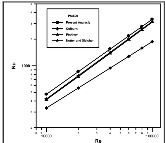
Figure (9) Comparison between Nu Obtained from Present Analysis with Other Works at Pr=600..
