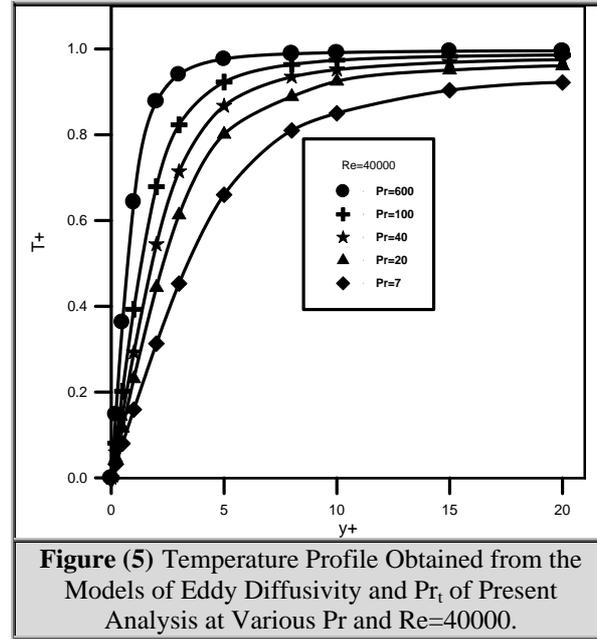
Figure (5) Temperature Profile Obtained from the Models of Eddy Diffusivity and  $\text{Pr}_t$  of Present Analysis at Various  $\text{Pr}$  and  $\text{Re}=40000$ .
