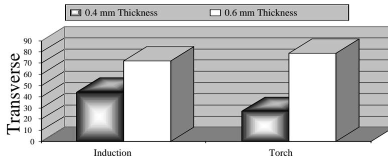
**Figure (2): Effect of interaction between casting technique and thickness.**
