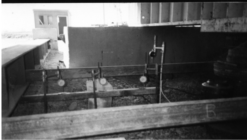
Plate (2) Positions of Points of dir.2 (4,5,and6) orthogonal to reference beam of 18m long
