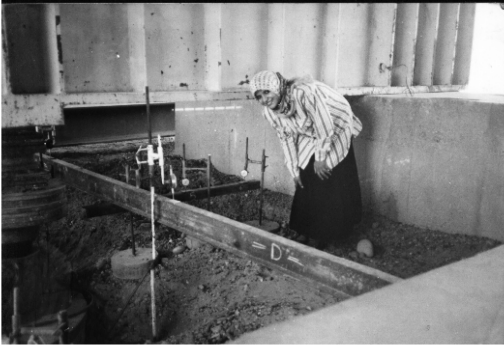
Plate-3-. Soil neighboring pile body effected by loading system after finishing the test
