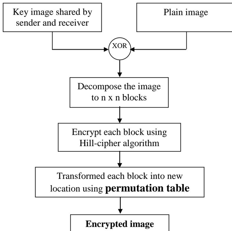
Fig. (1) Block diagram of the proposed algorithm
