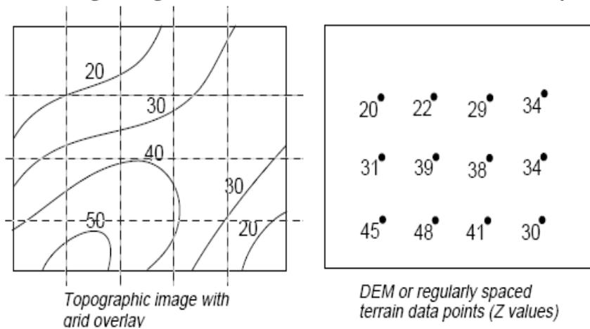
**Fig .4a. Regularly Spaced Terrain Data Points**
