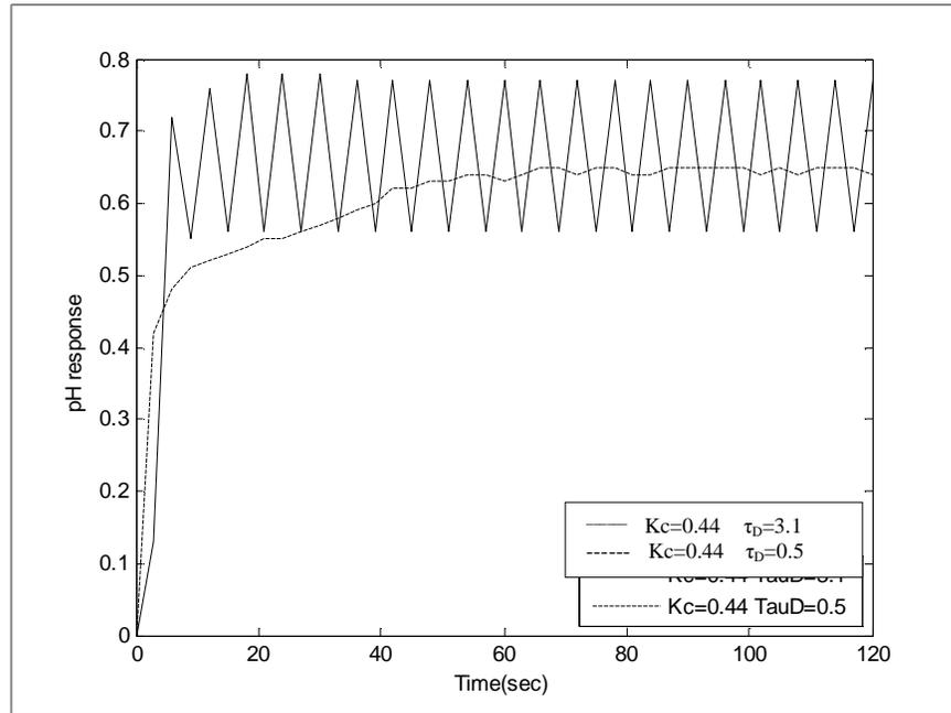
Figure (9-a): pH Response for PD-Control.
