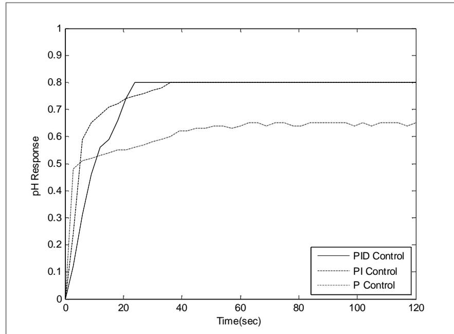
Figure (12): pH Response for Different Control Modes.
