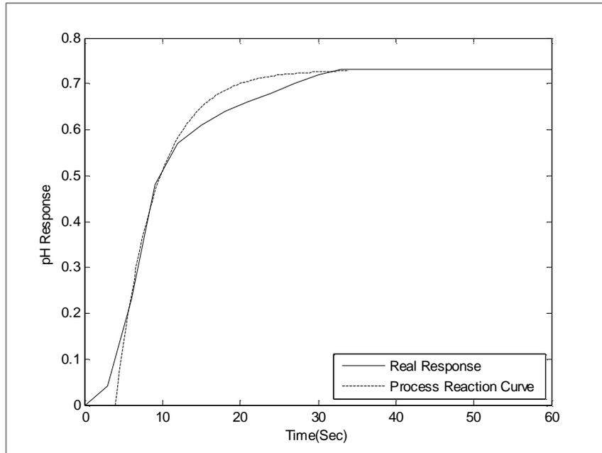
Figure(6-a): Open Loop Response Against +ve 10% Step Change in  $\text{Ca}(\text{OH})_2$  Flow Rate Solution.
