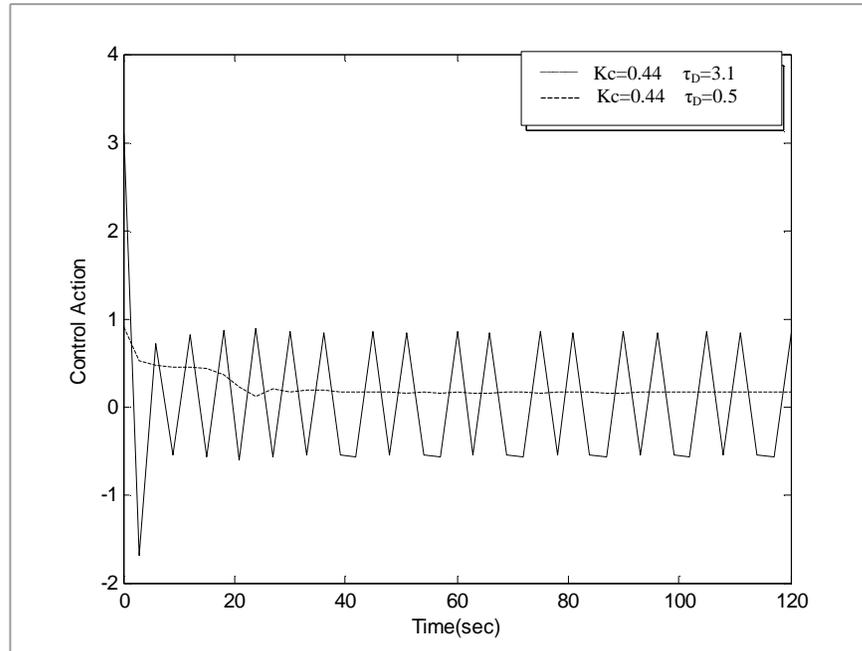
Figure (9-b): Control Action for PD-Control.
