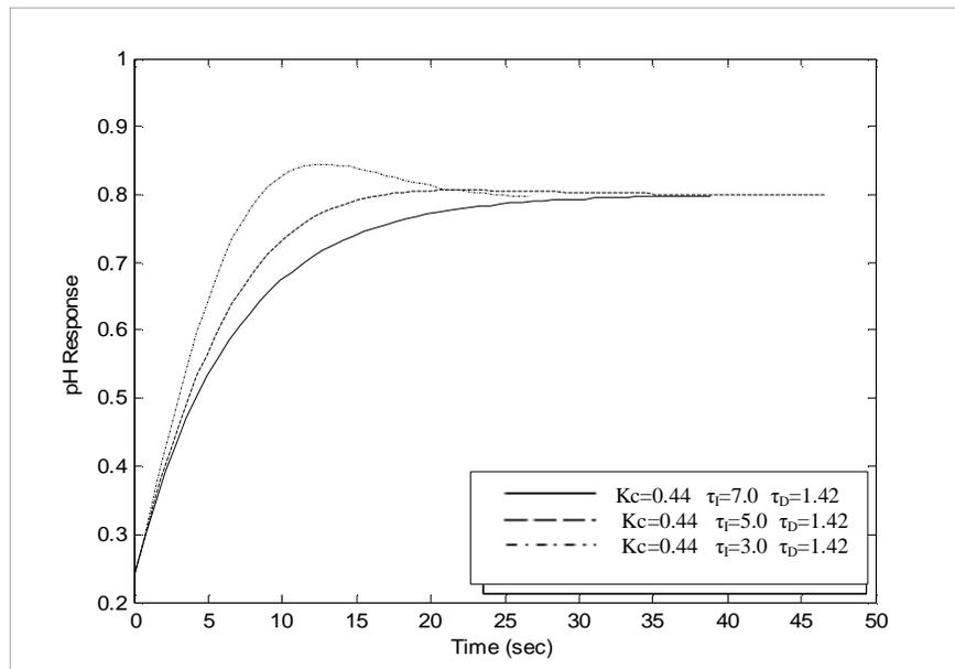
Figure (11): pH Response for PID-Control for Various Values of  $\tau_i$ .
