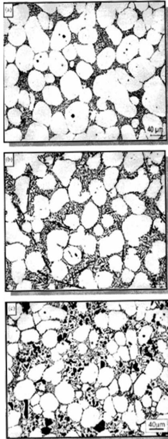
**Fig.(3):** Microstructure (a-c) of thixoformed Alloys (Alloys 4-6).
