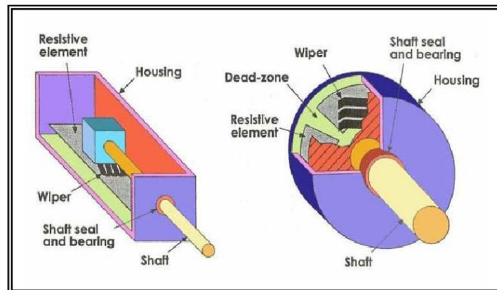
**Fig. (1):** Commonly termed potentiometers or “pots” <sup>(3)</sup>.
