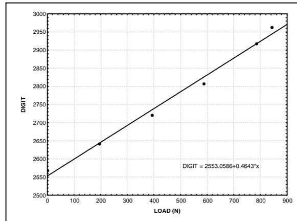
**Fig.(11):** The applied load-digit relation.
