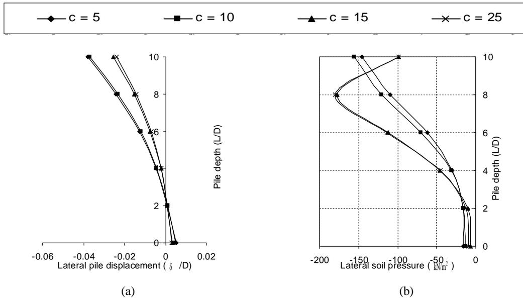
**Fig. (3):** Influence of the value of cohesion intercept values on the lateral pile response, (a) lateral pile displacement and (b) Lateral soil pressure.
