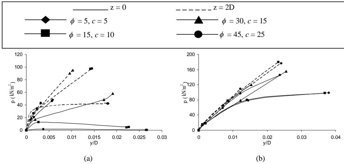
Fig.( 4): p-y curves predicted under the effect of soil properties,
