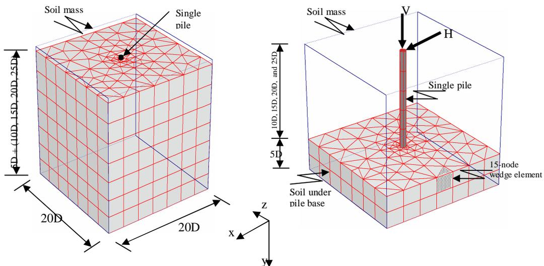
**Fig.(1):** Three dimension finite element mash for single pile and surrounded soil mass.
