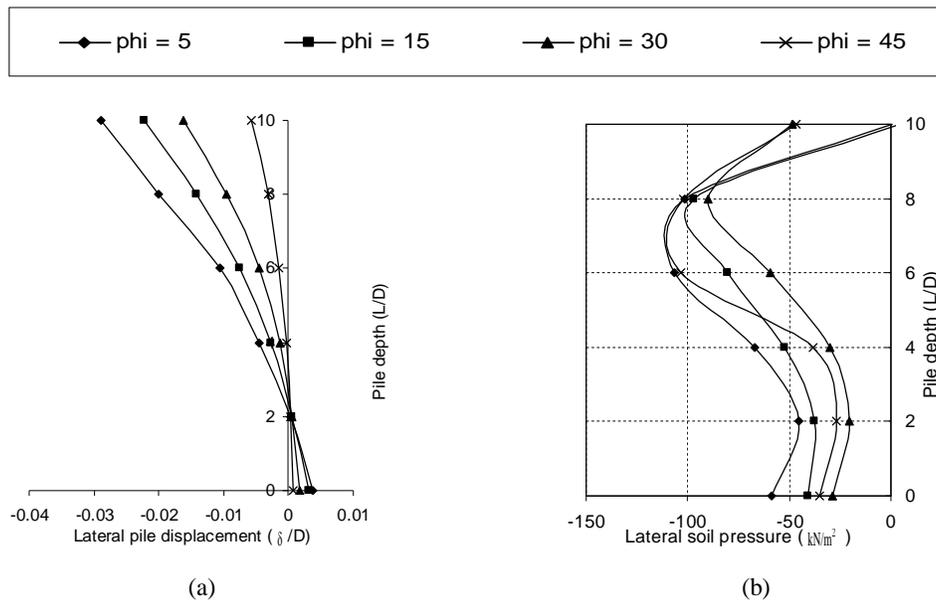
**Fig.(2):** Influence of the value of angle of internal friction on the lateral pile response, (a) lateral pile displacement and (b) Lateral soil pressure.
