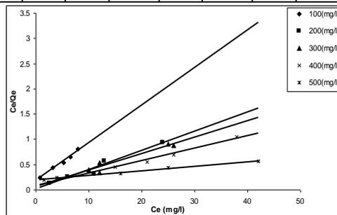
**Fig 3:** Langmuir isotherms of  $Pb^{2+}$  adsorption on bentonite .
