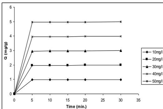
**Fig 1:** Effect of contact time on the adsorption amount.
