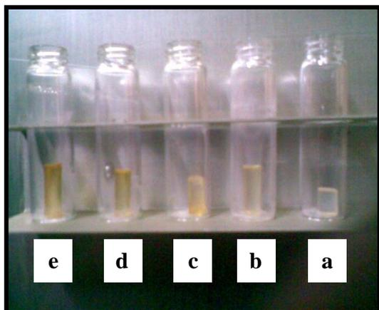
**Fig. 2:** Photographs of transparent monoliths with different Sm content, (a) non-doped, (b) 0.01M (c) 0.05M , (d) 0.1M and (e) 0.5 M
