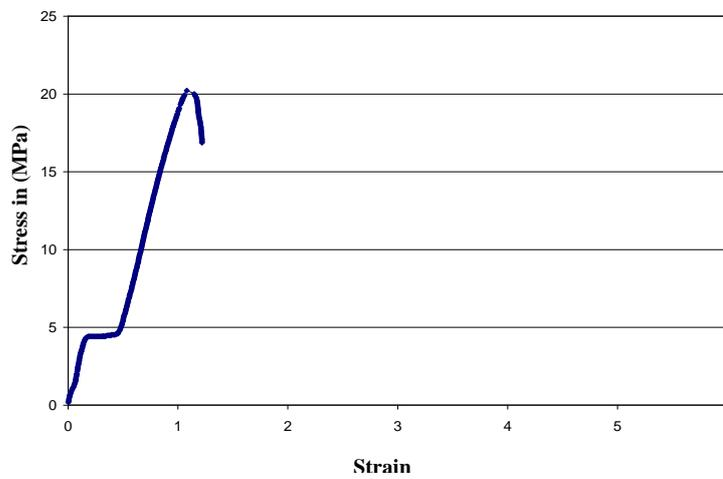
Fig. (8) Stress strain curve of Sample (AS29) Atomization pressure =8 mbar distance from nozzle =12 cm.
