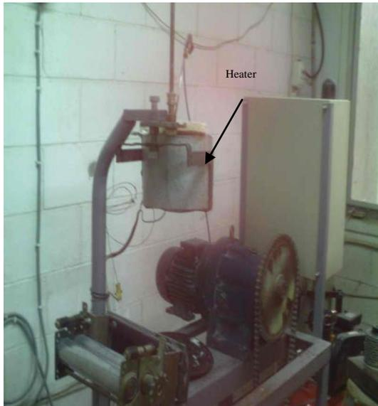
Fig. (1) The atomization apparatus used in preparation.
