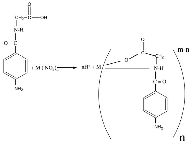
As indicated from the above figure. Bonding may occur through oxygen atom of the carboxylate ion and the lone pair electrons of the amide nitrogen atom.
