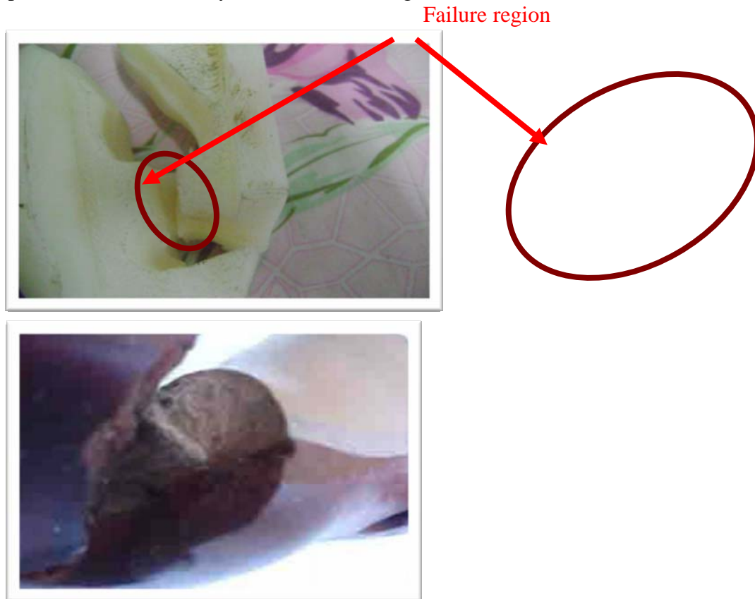
Fig. 8 Failure region in New foot and SACH foot.
