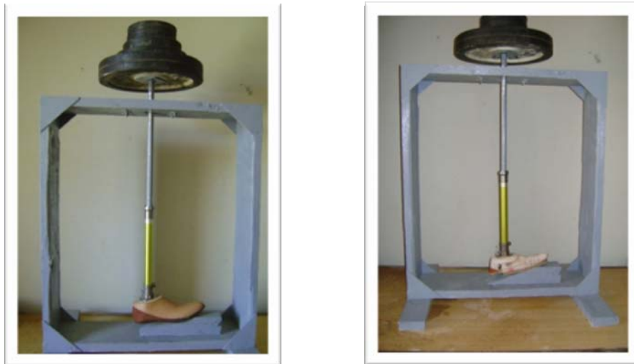
Fig. 5 Dorsiflexion tester of SACH foot and NEW foot.
