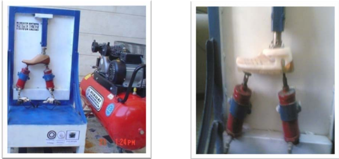
Fig. 4 Fatigue foot tester of SACH foot and NEW foot.
