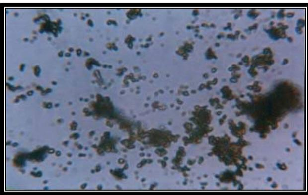
Figure (5) Photomicrograph of scales from heater surface without magnetic field
