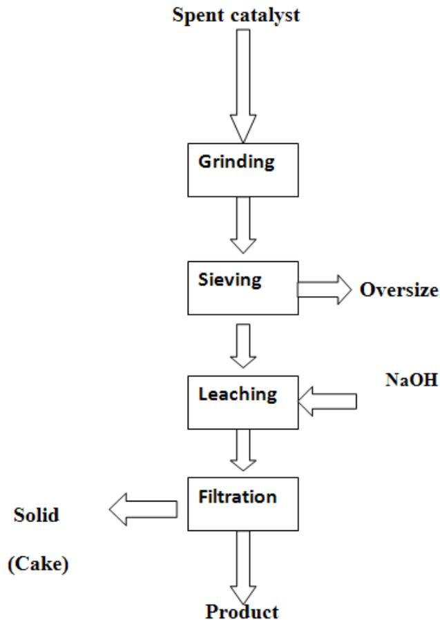
Fig.2. Experimental Procedure Block Diagram
