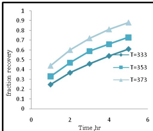
Fig. 7 effect of time on vanadium fraction recovery for 65 mesh size and 4 molar NaOH
