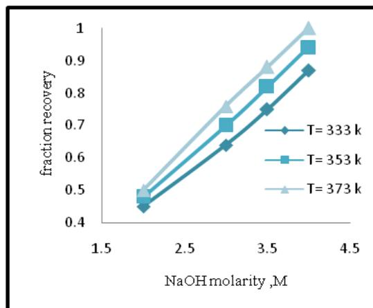
Fig. 6: Effect of NaOH molarity on vanadium fraction recovery for 5 h and 150 mesh size.
