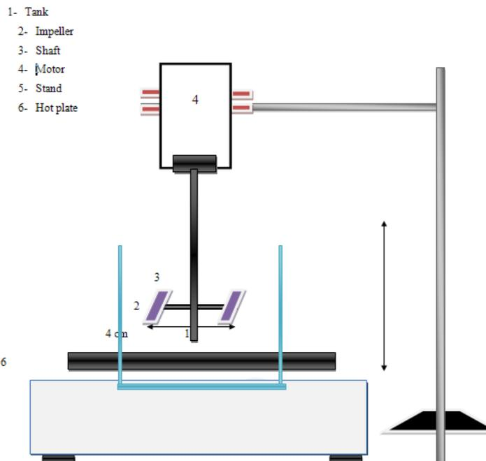
Fig. 1 A schematic Diagram of the Reactor system
