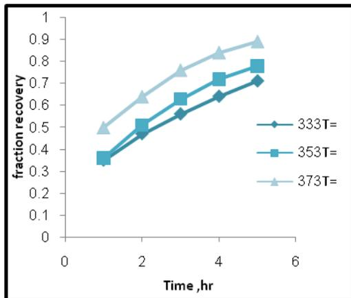
Fig. 8 effect of time on vanadium fraction recovery at different temperatures for 100 mesh size and 4 molar NaOH.
