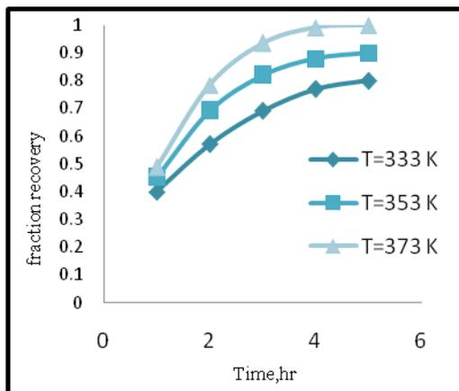
Fig. 9 effect of time on vanadium fraction recovery for 150 mesh size and 4 molar NaOH
