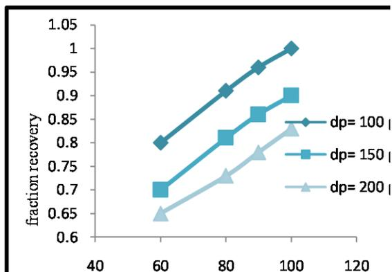
Fig. 4 Effect of temperature on vanadium fraction recovery at different time for 3 molar and 150 mesh sizes
