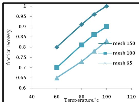
Fig 5 Effect of temperature on vanadium fraction recovery for 4 molar and 5 h
