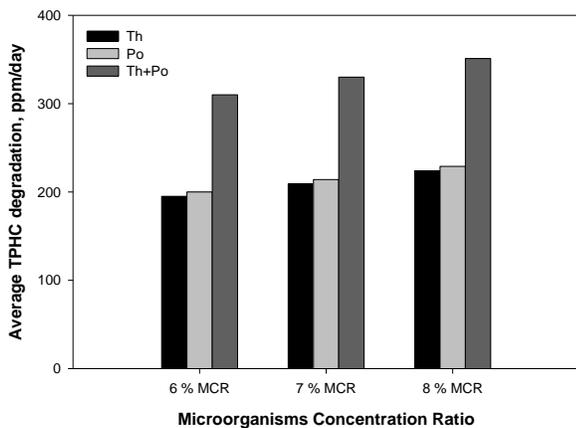
Fig. 4 Average hydrocarbon degradation response to both fungi stains and ratios with 8 % NWR and C/N/P=35/10/1, C/K=10
