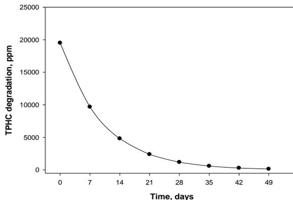
Fig. 6 Hydrocarbon degradation over time during the biotreatment of diesel contaminated soil at 8 % MCR, 8 % NWR and C/N/P=100/60/10, C/K=10
