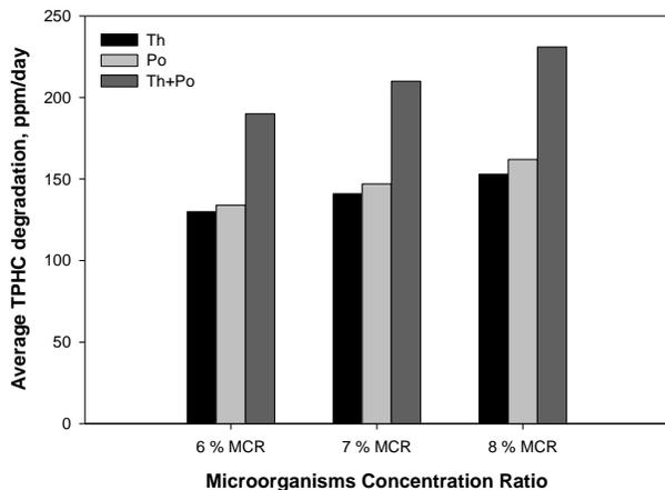
Fig. 1 Average hydrocarbon degradation response to both fungi strains and ratios without nutrients
