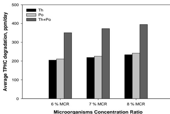
Fig. 5 Average hydrocarbon degradation response to both fungi stains and ratios with 8 % NWR and C/N/P=100/60/10, C/K=10
