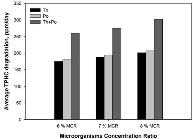
Fig. 2 Average hydrocarbon degradation response to both fungi stains and ratios with 6 % NWR and C/N/P=35/10/1
