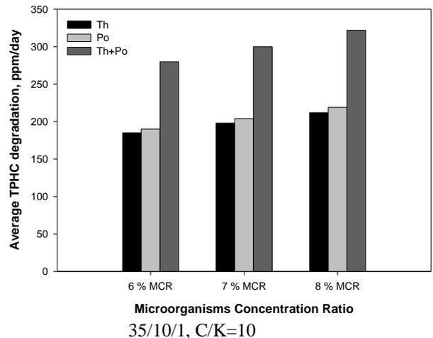
Fig. 3 Average hydrocarbon degradation response to both fungi strains and ratios with 6 % NWR and C/N/P=100/60/10, C/K=10
