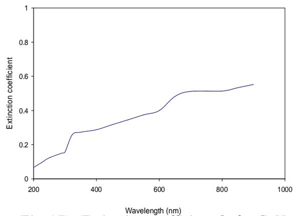
Fig. (7) Extinction coefficient  $k$  for GaN thin film
