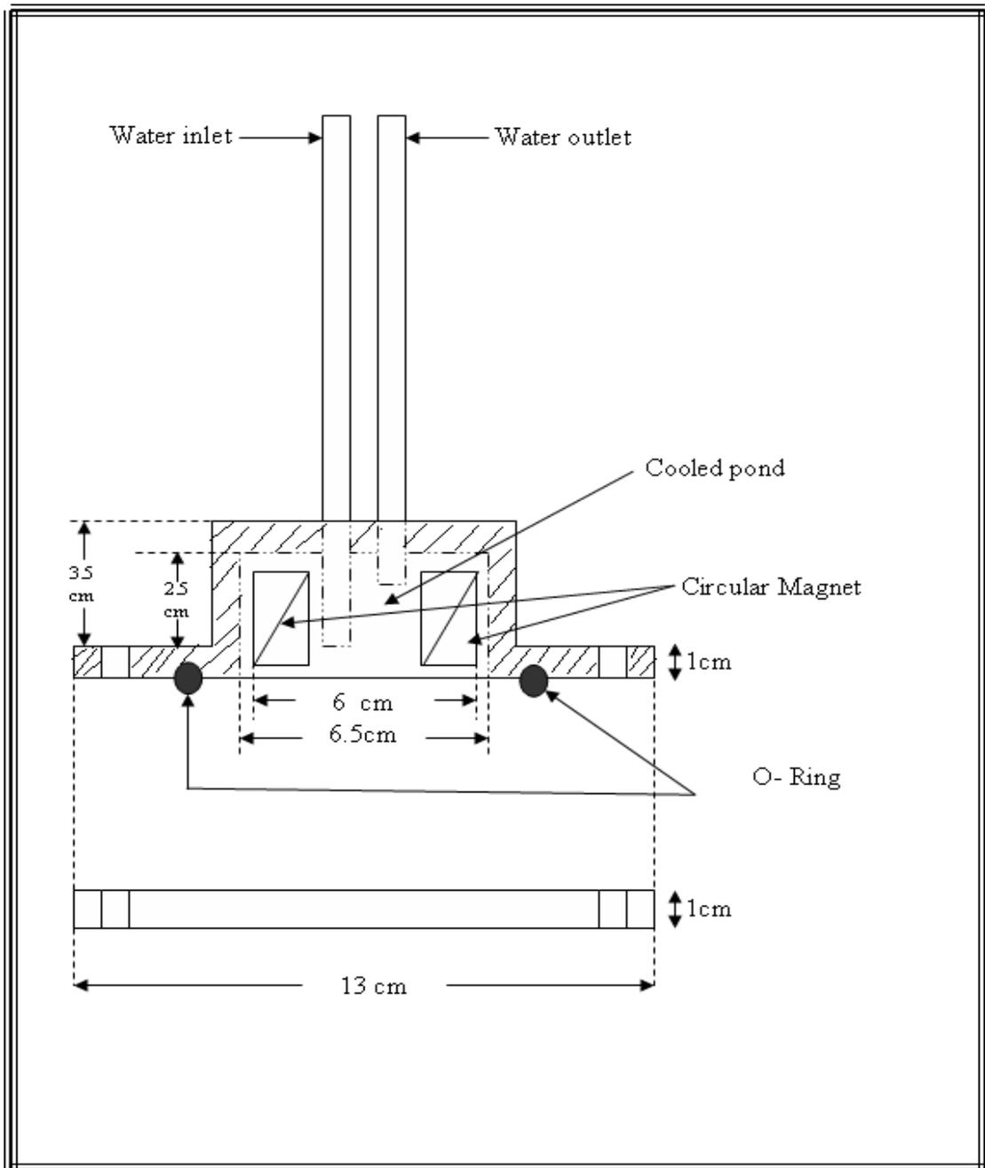
Figure (5) the target diagram
