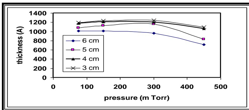
**Figure (7) The variation of film thickness of a function of pressure**
