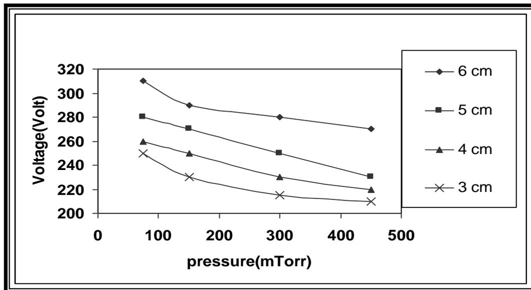
Figure( 6) The variation of target voltage as a function of pressure of different distance.
