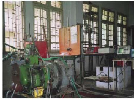
Fig. 1, Ricardo engine and its accessories used in this study
