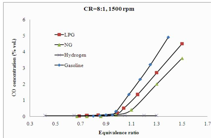
Figure 4, CO concentrations for wide range of equivalence ratios for the four fuels used in research at CR=8:1
