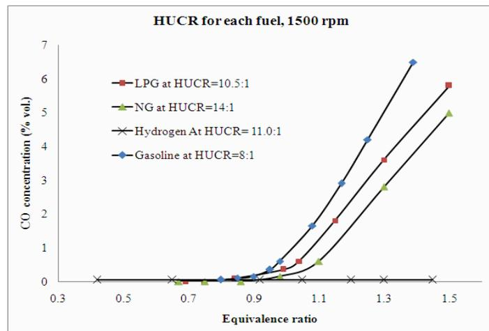
Figure 5, CO concentrations for wide range of equivalence ratios for the four fuels used in research at HUCR for each fuel and 1500 rpm engine speed (medium speed)
