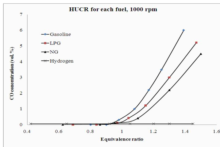
Figure 6, CO concentrations for wide range of equivalence ratios for the four fuels used in research at HUCR for each fuel and 1000 rpm engine speed (low speed)
