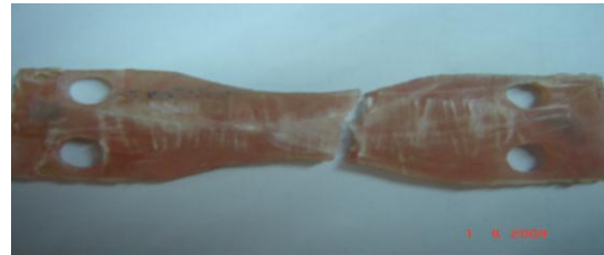
Fig(4): Photographic pictures for wet PMMA reinforced with woven glass fiber
