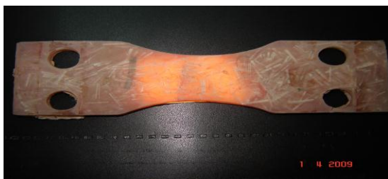
Fig(2): Photographic pictures for wet PMMA reinforced with chopped glass fiber
