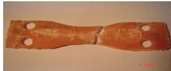
Fig(5): Photographic pictures for dry PMMA reinforced with woven glass fiber
