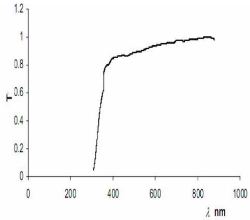
Fig.(3):The spectral transmission(T)As afunction of wavelength( $\lambda$ )
