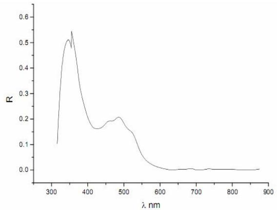
Fig. (7):Reflectance (R)as a function of wavelength( $\lambda$ )
