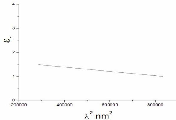
Fig. ( 12 ):Real part of dielectric constant (ε<sub>r</sub>)as a function of square of wavelength (λ<sup>2</sup>)
