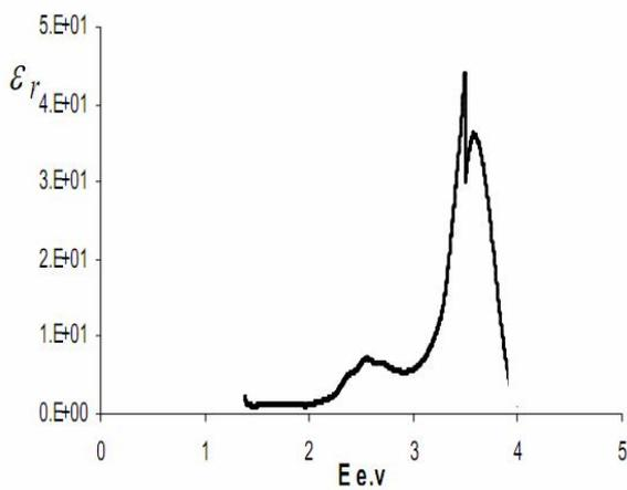
Fig. ( 10): Real part of dielectric constant(ε<sub>r</sub>) as a function of photon energy(E)
