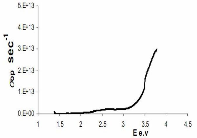
Fig. ( 9): Optical conductivity(σ<sub>op</sub>)as a function of photon energy(E)
