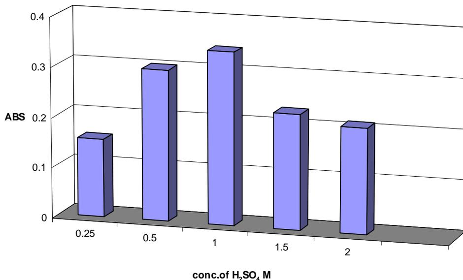
**Fig. 2: Effect of H<sub>2</sub>SO<sub>4</sub> concentration on the Absorbance measurements of 80 µg.ml<sup>-1</sup> tetracycline in presence of 2.5x10<sup>-3</sup> M Ce(IV) solution .**
