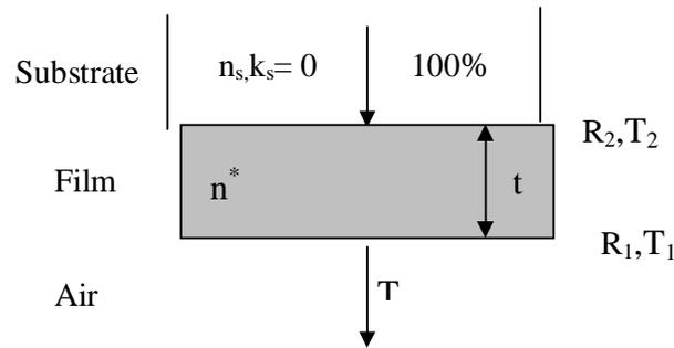
**Fig.1 Schematic diagram film-substrate system**
