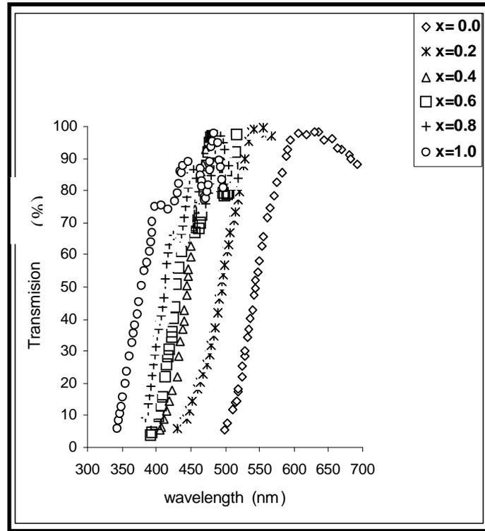
**Fig.2: Transmission spectra of films with different Zn concentration**
