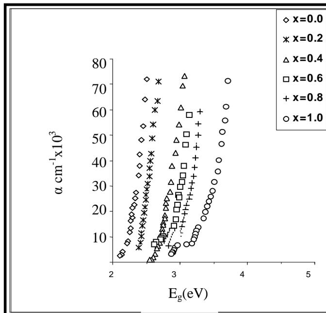
**Fig.3: absorption coefficient versus photon energy of films with different Zn concentration**
