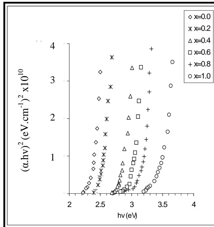
**Fig.4: (αhν)<sup>2</sup> versus hν plot of thin films with different Zn concentration**
