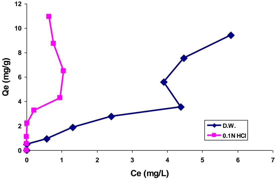
Figure (2): Adsorption isotherms of metronidazole in distilled water (D.W.) and 0.1N HCl on bentonite surface at 25°C.
