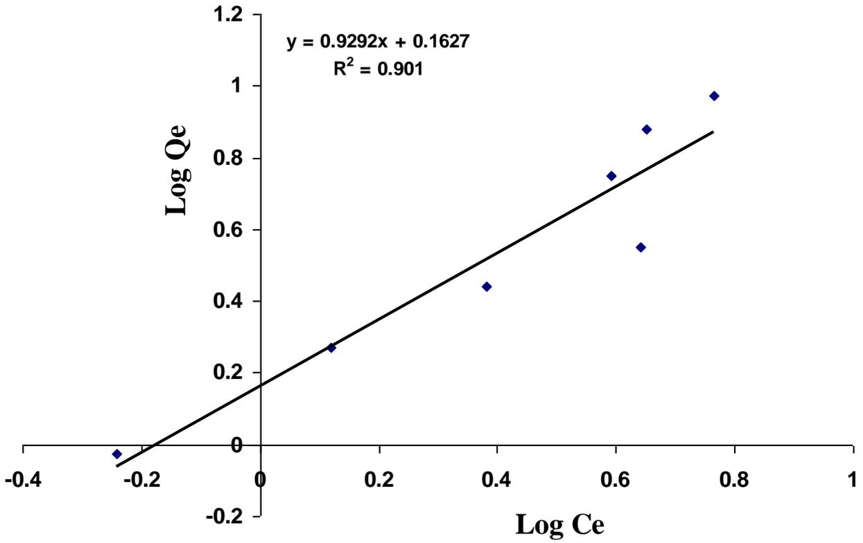
Figure (1): Linear form of Freundlich equation for the adsorption of metronidazole on bentonite. Fi
