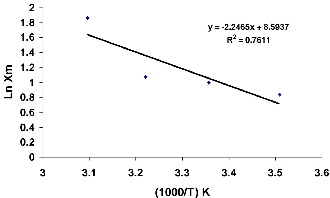
Figure (4):Graphic representation of the modified vantHoff's equation for the adsorption of metronidazole on bentonite at different temperatures.
