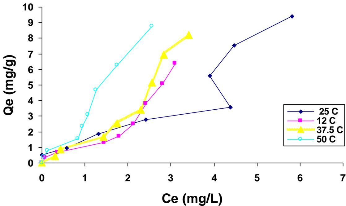
Figure (3): Adsorption isotherm of metronidazole on bentonite surface at (12, 25, 37.5, and 50°C)
