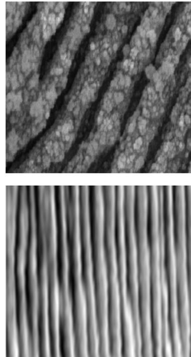
Fig. (2) The periodic structured of the irradiated cell, by a 100fs laser pulses, 800nm wavelength, 4μm length (above) and 12μm length (below)
