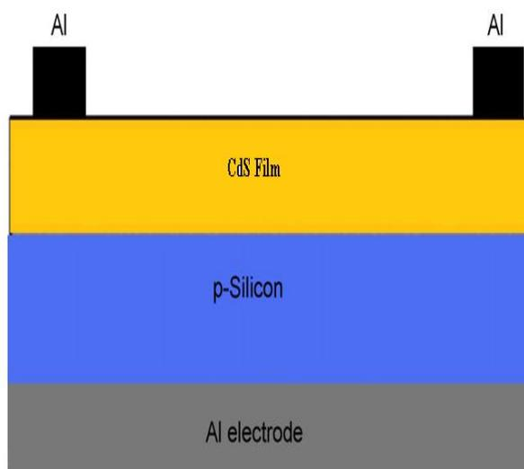
Figure (1): The schematic diagram of the CdS/p-Si heterojunction detector.
