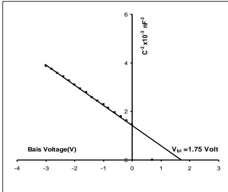
Fig.(7)  $C^{-2}$  versus Bias voltage for characteristics CdS/Si heterojunction.
