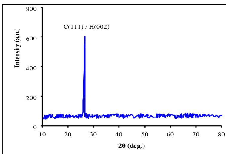
Figure (2): The X-ray diffraction patterns of CdS thin films.
