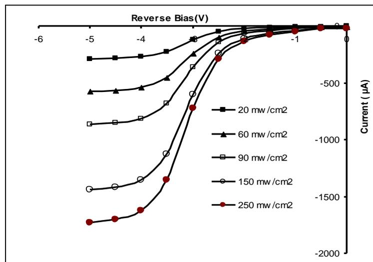
Fig. (6) Current-voltage in illumination condition for characteristics CdS/Si heterojunction.
