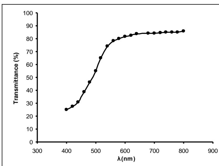
Figure (3): The optical transmission spectra as a function of wavelength of CdS thin films
