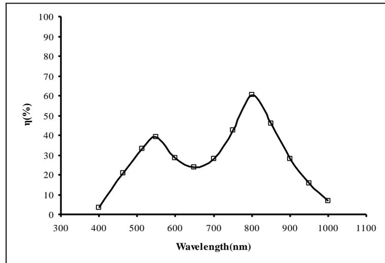
Fig. (9) quantum efficiency as a function of wavelength of CdS /Si Detector.
