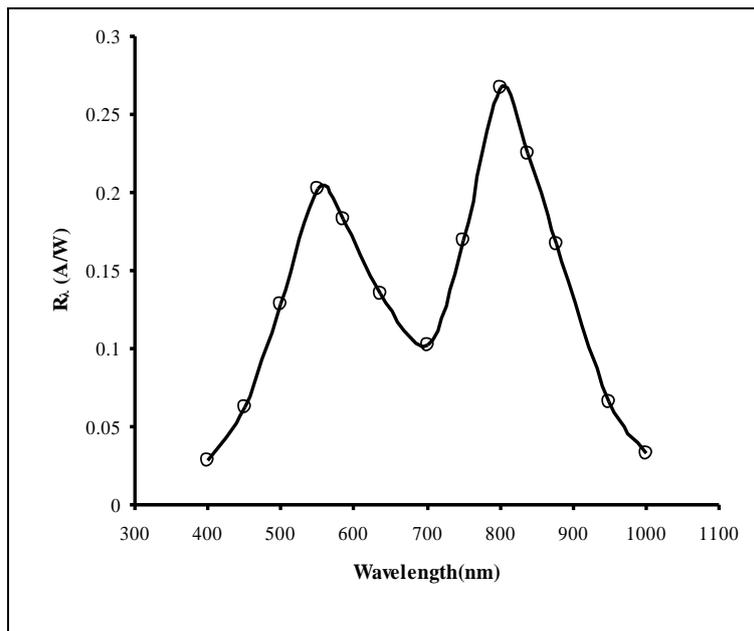
Fig. (8) responsivity as a function of the wavelength of CdS /Si Detector.
