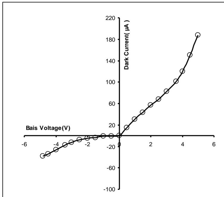
Fig. (5) current-voltage for characteristics CdS/Si heterojunction.
