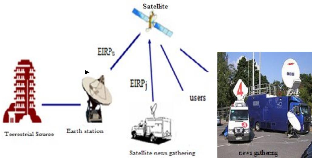
Figure 4. The method of jamming by using Satellite news gathering<sup>[8]</sup>.
