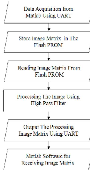
**Figure 3** block diagram of the application program
