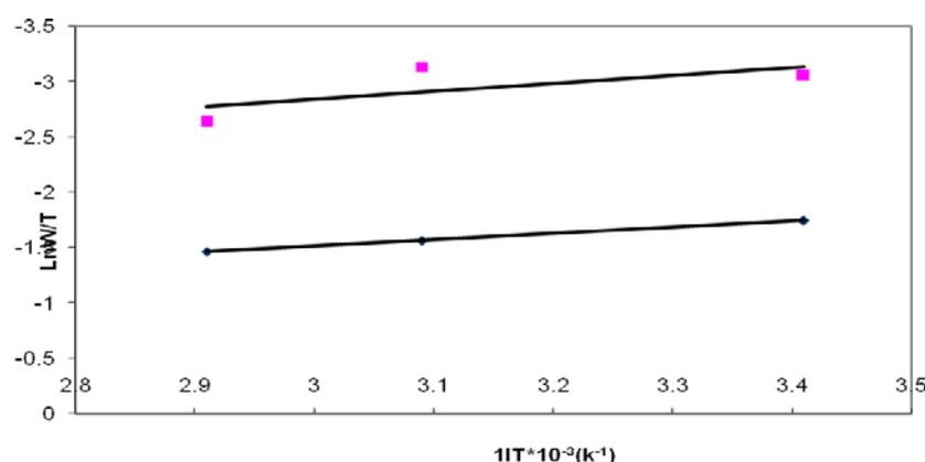
Fig. 18: Arrhenius plots of  $\ln w/T$  Vs  $1/T$  1N HCL  $\blacklozenge$  without inhibitor  $\blacksquare$  with 10ppm inhibitor
