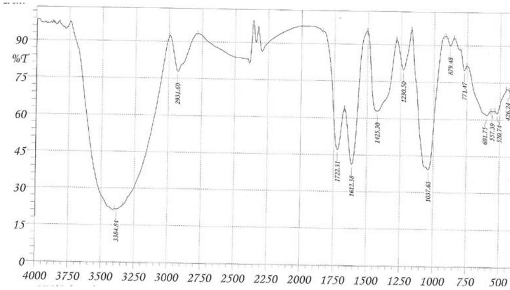
**Fig. 19: FT-IR spectra of pomegranate shells extract**
