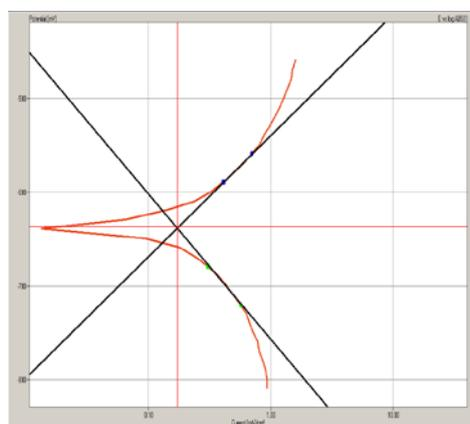
**Fig. 3.** Polarization curves for C- steel in 1N HCl at 343 k° .
