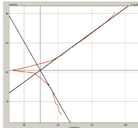
**Fig. 10.** Polarization curves for C-Steel 1N HCl containing 10 ppm pomegranate shells extracts at 293 k° .
