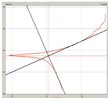
**Fig. 1.** Polarization curves for C- steel in 1N HCl at 293 k° .
