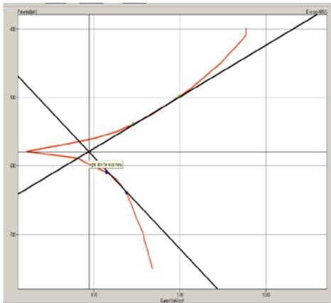
**Fig. 9.** Polarization curves for C- steel in 1N HCl containing 5 ppm pomegranate shells extracts at 343 k° .
