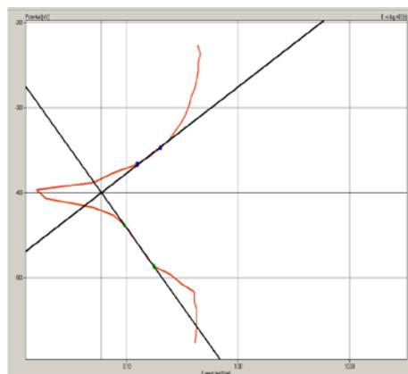
**Fig. 5.** Polarization curves for C- steel in 1N HCl containing 1 ppm pomegranate shells extracts at 323 k° .
