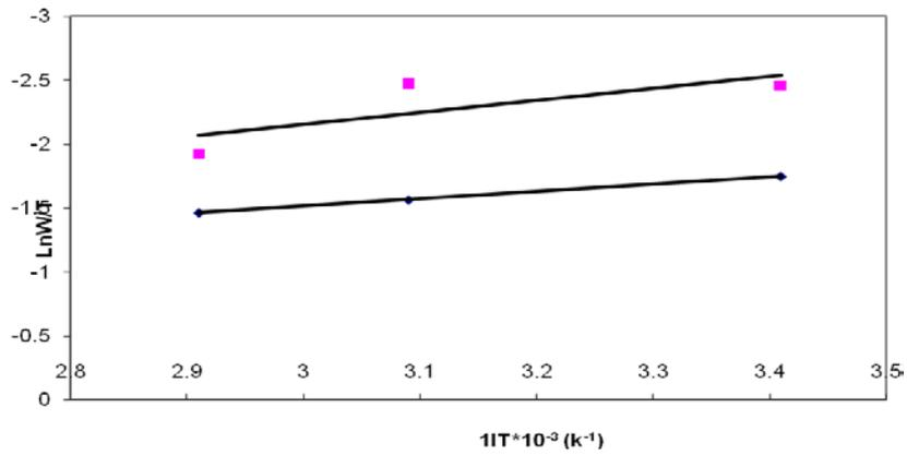
**Fig.16:** Typical Arrhenius plots of  $\ln w/T$  Vs  $1/T$  1N HCl  $\blacklozenge$  without inhibitor  $\blacksquare$  with 1ppm inhibitor
