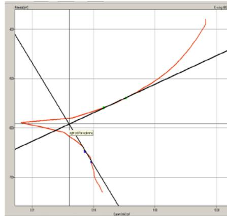
**Fig. 8.** Polarization curves for C- steel in 1N HCl containing 5 ppm pomegranate shells extracts at 323 k° .
