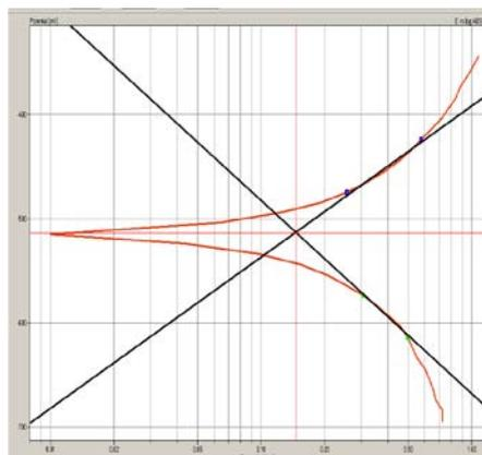
**Fig. 2.** Polarization curves for C- steel in 1N HCl at 323 k° .
