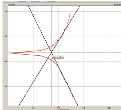
**Fig. 6.** Polarization curves for C- steel in 1N HCl containing 1 ppm pomegranate shells extracts at 343 k° .
