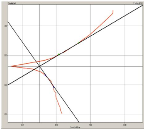
**Fig. 7.** Polarization curves for C- steel in 1N HCl containing 5 ppm pomegranate shells extract at 293 k° .
