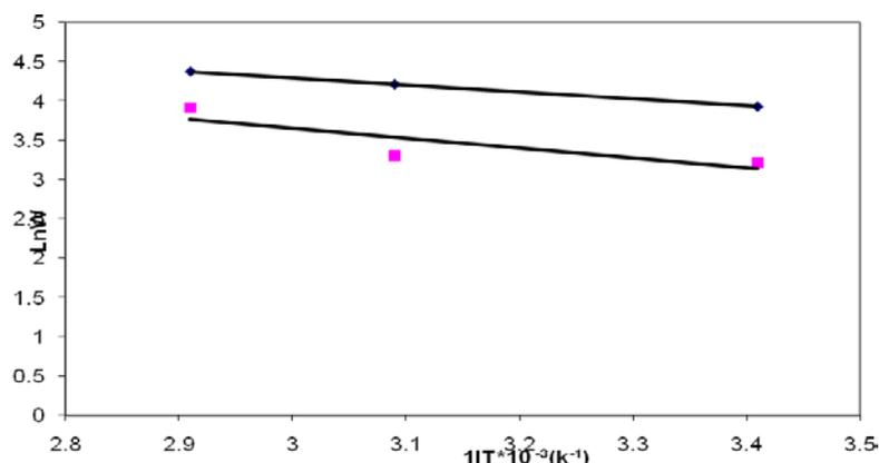
Fig. 13: Typical Arrhenius plots of  $\ln w$  Vs  $1/T$  in 1N HCl  $\blacklozenge$  control  $\blacksquare$  with 1ppm inhibitor
