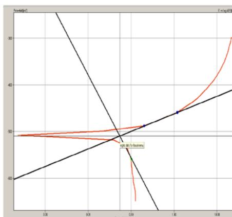
**Fig. 4.** Polarization curves for C- steel in 1N HCl containing 1 ppm pomegranate shells extracts at 293 k° .
