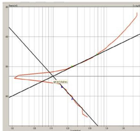
**Fig. 12.** Polarization curves for C- steel in 1N HCl containing 10 ppm pomegranate shells extracts at 343 k° .
