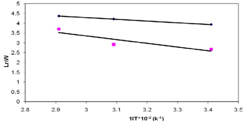
**Fig. 14:** Arrhenius plots of  $\ln w$  Vs  $1/T$  at 1N HCl  $\blacklozenge$  without inhibitor  $\blacksquare$  with 5ppm inhibitor
