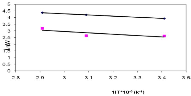
**Fig. 15:** Arrhenius plots of  $\ln w$  Vs  $1/T$  at 1N HCl  $\blacklozenge$  without inhibitor  $\blacksquare$  with 10ppm inhibitor
