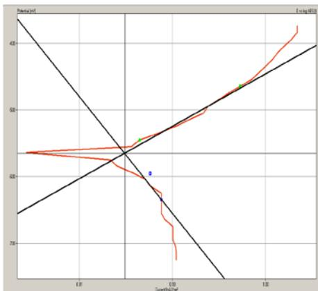
**Fig. 11.** Polarization curves for C-Steel in 1N HCl containing 10 ppm pomegranate shells extracts at 323 k° .
