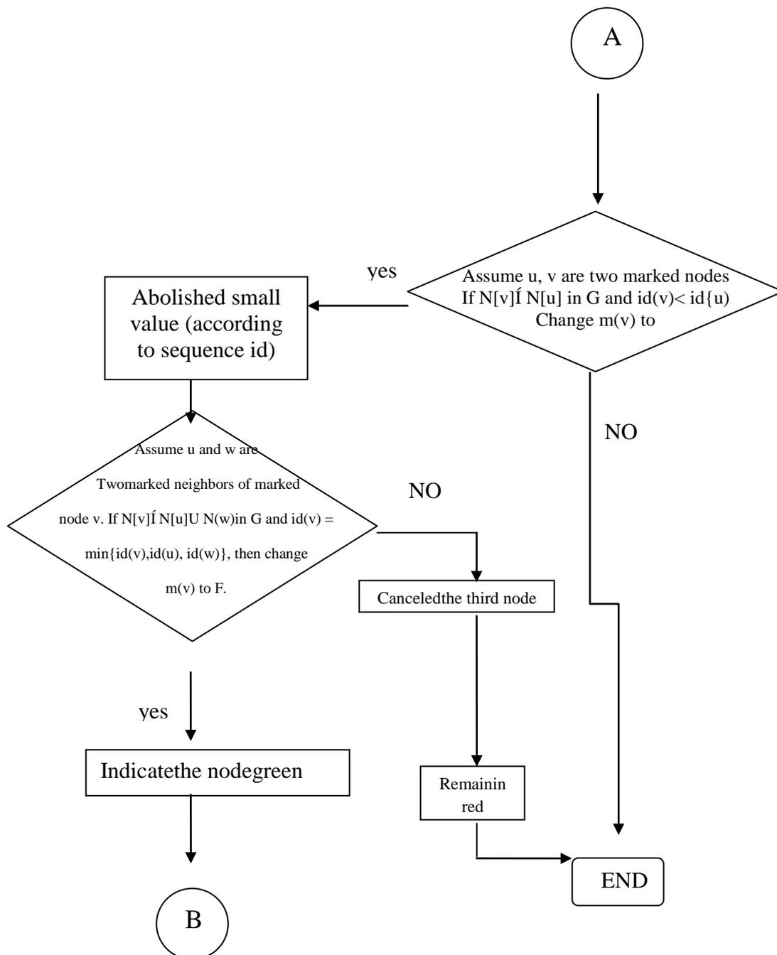
Figure 6. Flowchart to simulate the Wu & Li algorithm
