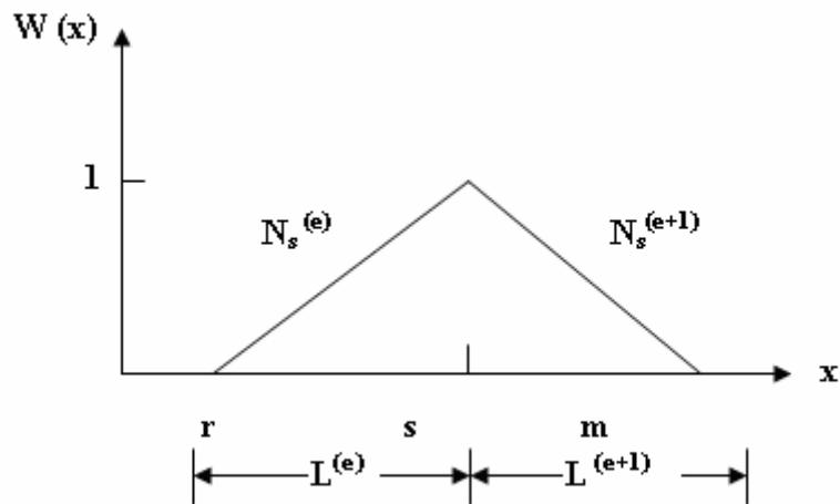
Fig.(2): The weighting function for an interior node [Segerlind].
