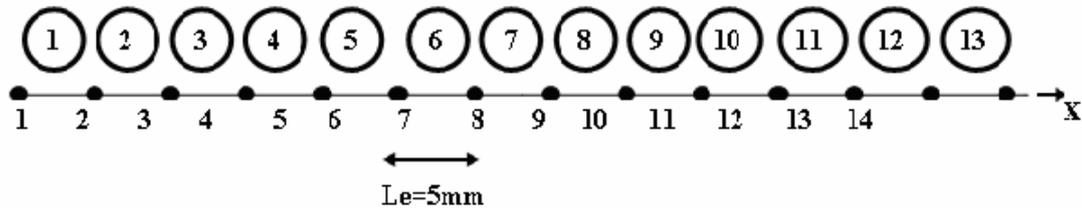
Fig.(1): Finite element mesh for flexural specimen
