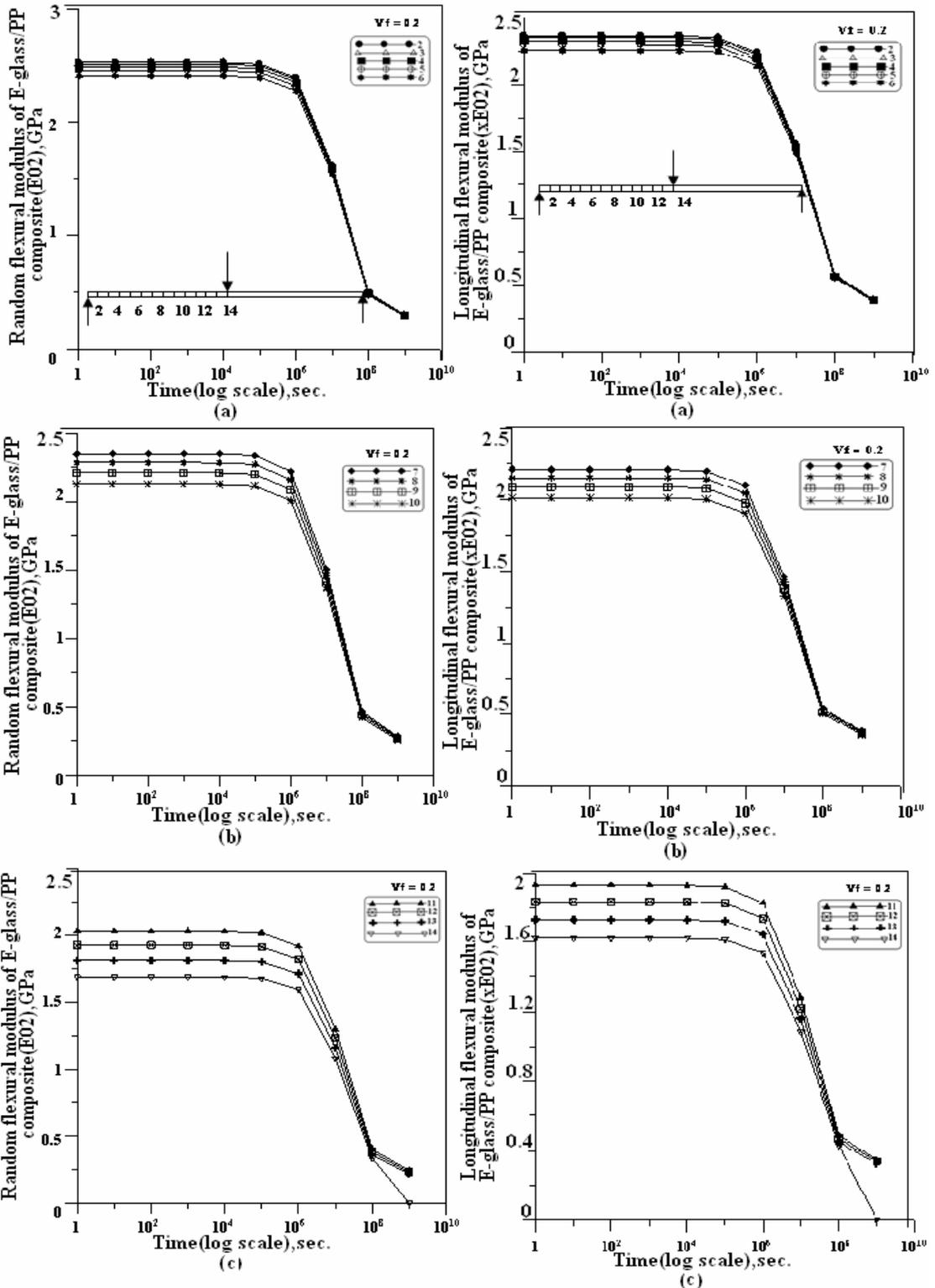
Fig.(7): Time dependent flexural modulus For random short E-glass/PP composite (Halpin-Tsai eq.) for nodes: a-(2-6);b-(7-10);c-(11-14)
