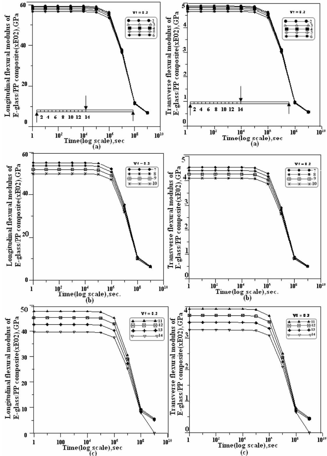
Fig.(5): Time dependent longitudinal flexural modulus for aligned short E-glass/PP composite(Halpin-Tsai eq.) for nodes: a-(2-6);b-(7-10);c- (11-14)
