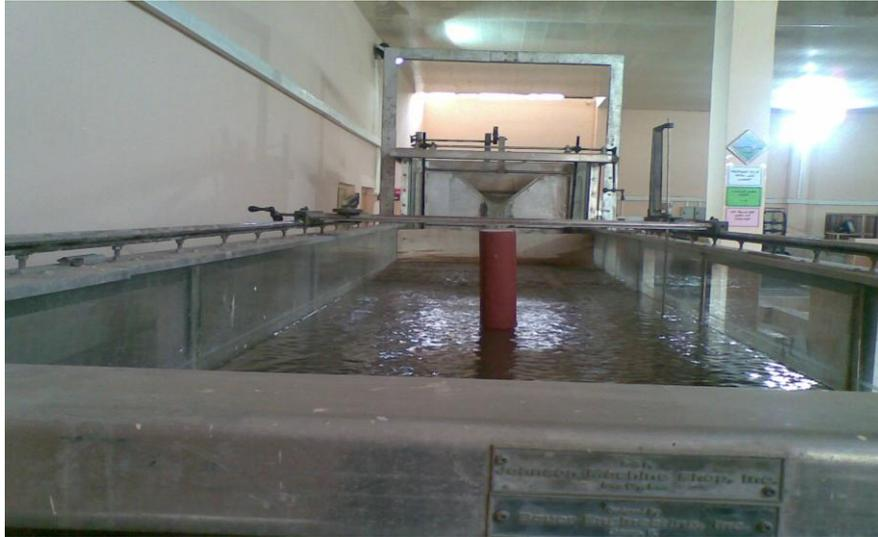
**Plate (1) General view of the laboratory flume with one of the piers.**
