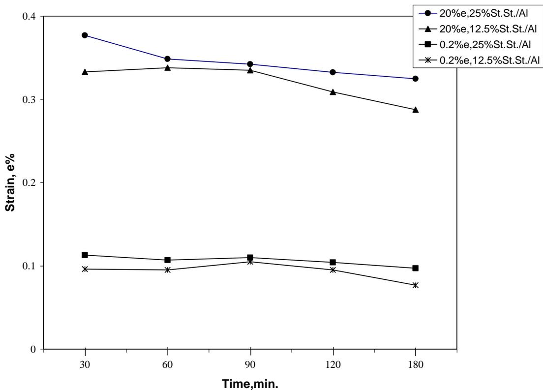
Fig. (4) Strain (work hardening) Vs sintering time, sintered at 900 °C.
