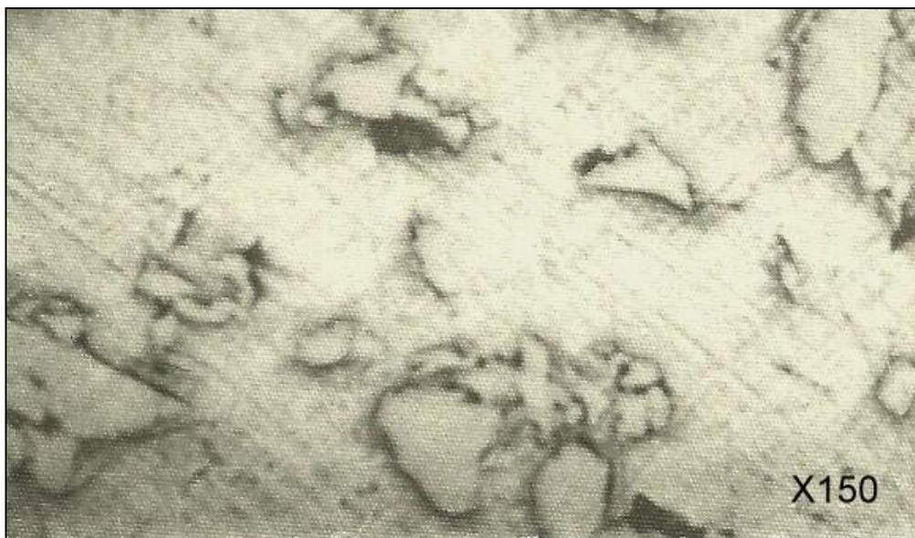
Fig.(f) The microstructure of the sintered specimen. The dark boundary islands are FeAl<sub>7</sub>.
