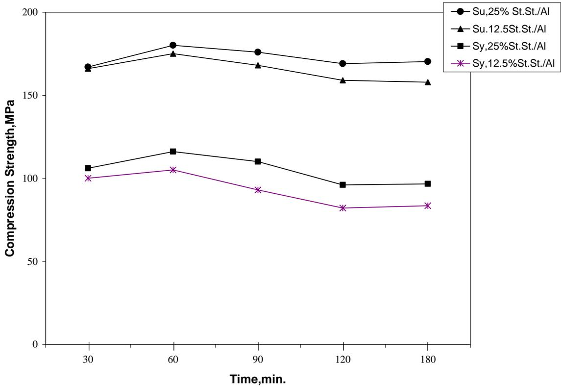
Fig. (1) Compression strength (Su) and yield strength (Sy) Vs sintering time, sintered at 530 °C.
