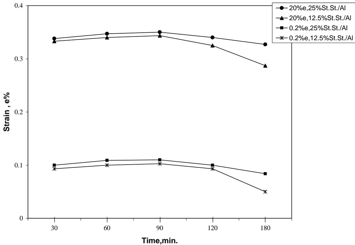
Fig. (3) Strain (work hardening) Vs sintering time, sintered at 930 °C.
