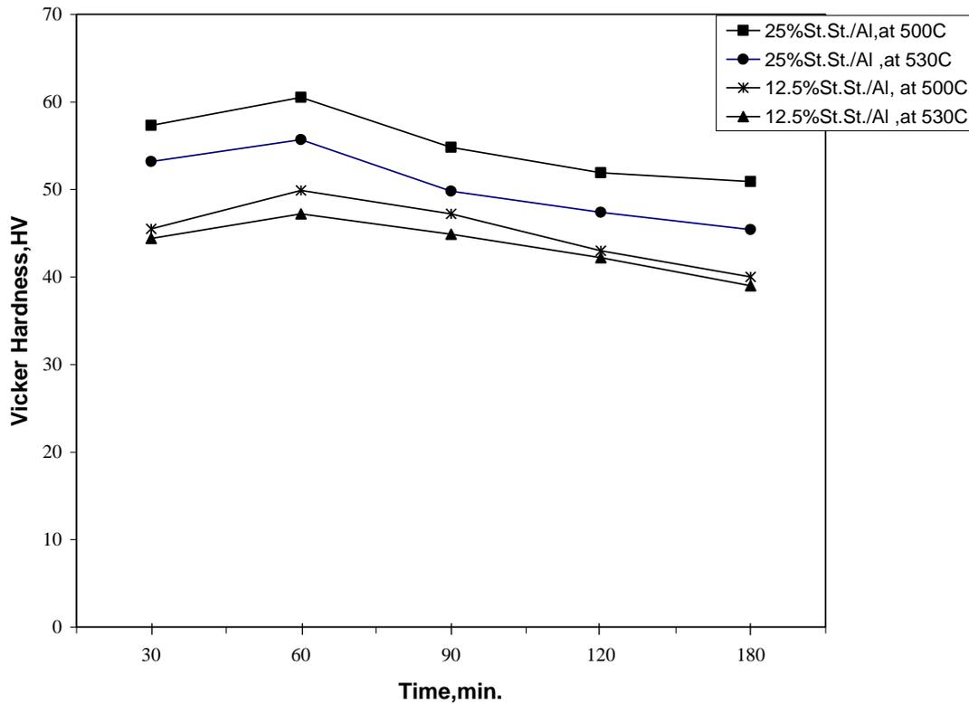
Fig. (e) Vicker Hardness Vs sintering time, sintered at 500 and 530 C.
