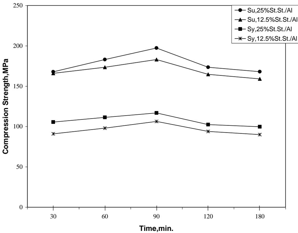
Fig. (2) Compression strength (Su) and yield strength (Sy) Vs sintering time, sintered at 500 °C.
