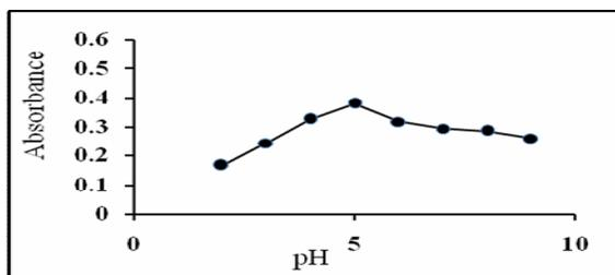
**Figure 4. Effect of pH on the formation of 7-(6-BrBTA8HQ)- Hg(II) complex . [ Conditions : Hg(II) = 0.2  $\mu\text{g mL}^{-1}$  , 0.45 ml of 7-(6-BrBTA8HQ) =  $3 \times 10^{-5}$  M , 0.2 mL of 10 % (v/v)Triton X-114 ]**
