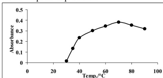
**Figure 7. Effect of the temperature on the absorbance for Hg(II) complex.** [ conditions : Hg(II) = 0.2  $\mu\text{g mL}^{-1}$ , 0.45 mL of 7-(6-BrBTA8HQ) =  $3 \times 10^{-5}$  M, 0.2 mL of 10 % (v/v) Triton X-114), pH 5.0 ].
