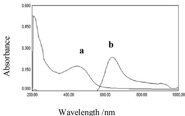
**Figure 2. Absorption spectra (a) Reagent 7-(6-BrBTA8HQ) =  $3 \times 10^{-5}$  M (b) Hg(II)- 7-(6-BrBTA8HQ) complex , Hg(II) =  $0.13 \mu\text{g mL}^{-1}$ , 0.45 ml of 7-(6-BrBTA8HQ) =  $3 \times 10^{-5}$  M , Buffer pH= 5( 1.5 mL ) , 0.2 mL of 10 % (v/v)Triton X-114 .**
