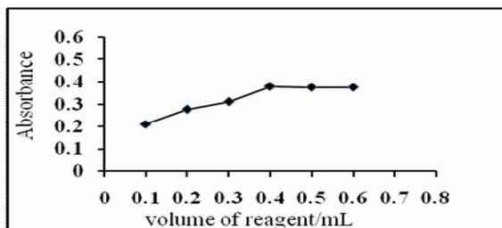
**Figure 5. Effect of concentration of 7-(6-BrBTA8HQ) on the Hg(II) analytical signal. [conditions : Hg(II) = 0.2  $\mu\text{g mL}^{-1}$  , X mL of 7-(6-BrBTA8HQ) =  $3 \times 10^{-5}$  M , 0.2 mL of 10 % (v/v)Triton X-114 , pH 5.0] .**
