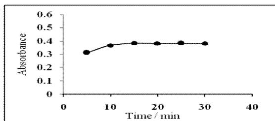
**Figure 8. Effect of the incubation time on the absorbance for Hg(II) complex.** [ conditions : Hg(II) = 0.2  $\mu\text{g mL}^{-1}$ , 0.45 mL of 7-(6-BrBTA8HQ) =  $3 \times 10^{-5}$  M, 0.2 mL of 10 % (v/v) Triton X-114), pH 5.0, temp 70 ° C].
