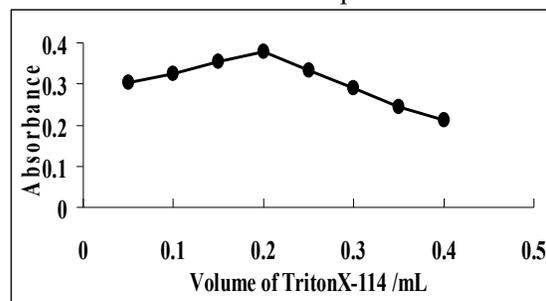
**Figure 6. Effect of Triton X-114 concentration on the Hg(II) analytical signal. [conditions : Hg(II) = 0.2  $\mu\text{g mL}^{-1}$  , 0.45 mL of 7-(6-BrBTA8HQ) =  $3 \times 10^{-5}$  M , X mL of 10 % (v/v)Triton X-114 , pH 5.0] .**
