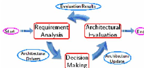
Fig 1. General s/w Architecture Design Method<sup>[10]</sup>
