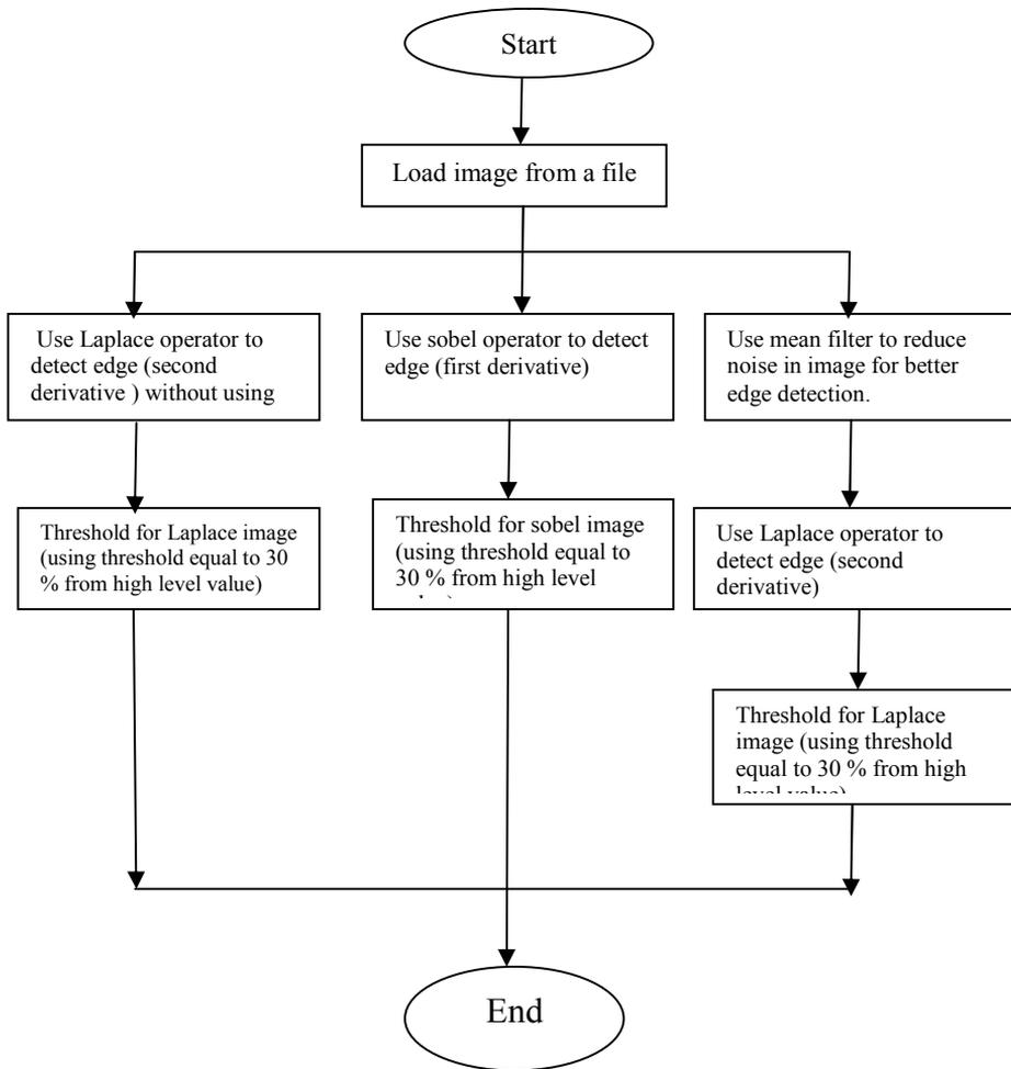
Figure.6 Block diagram of designed algorithm.
