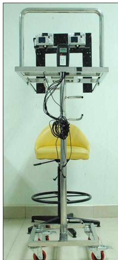
**Figure 1.** The complete imaging station from frontal view showing the camera base and remote control switch.
