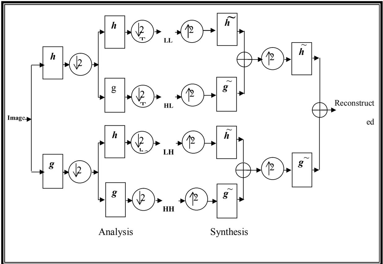
Figure (1): The analysis and synthesis of 2-D, 1-level discrete wavelet decomposition
