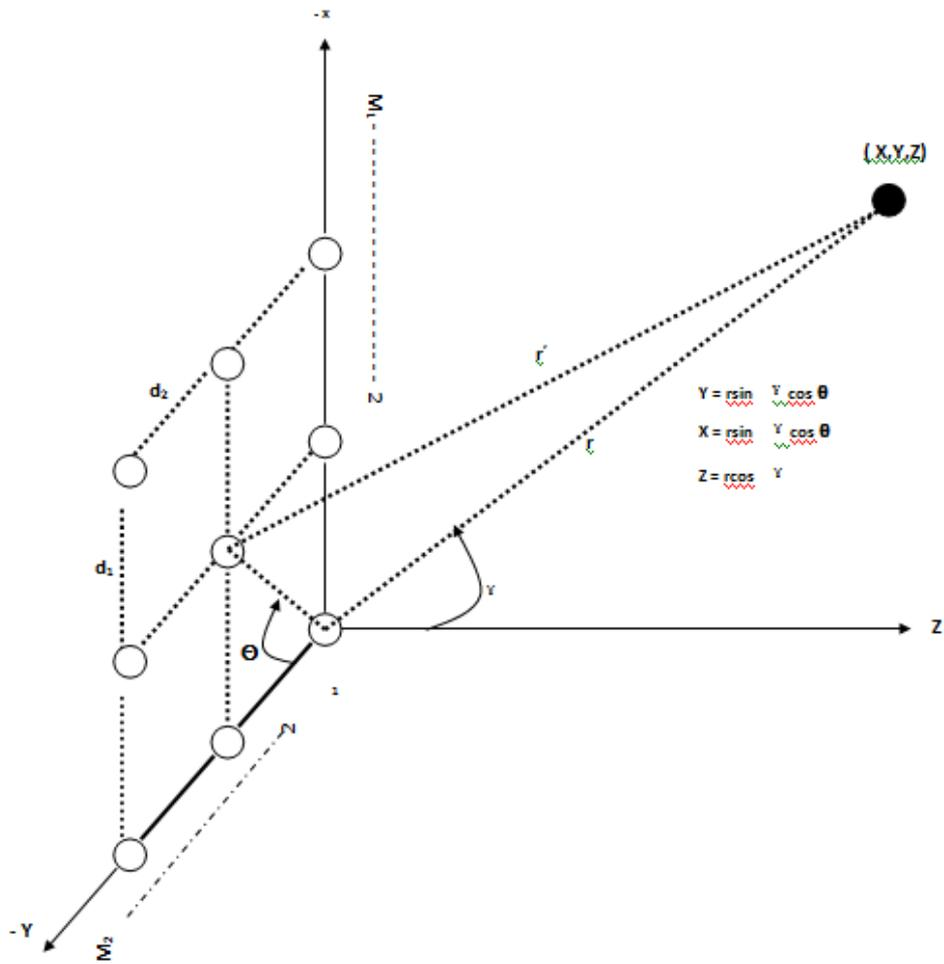
Figure -1 : The planner array geometry and the receiving signals
