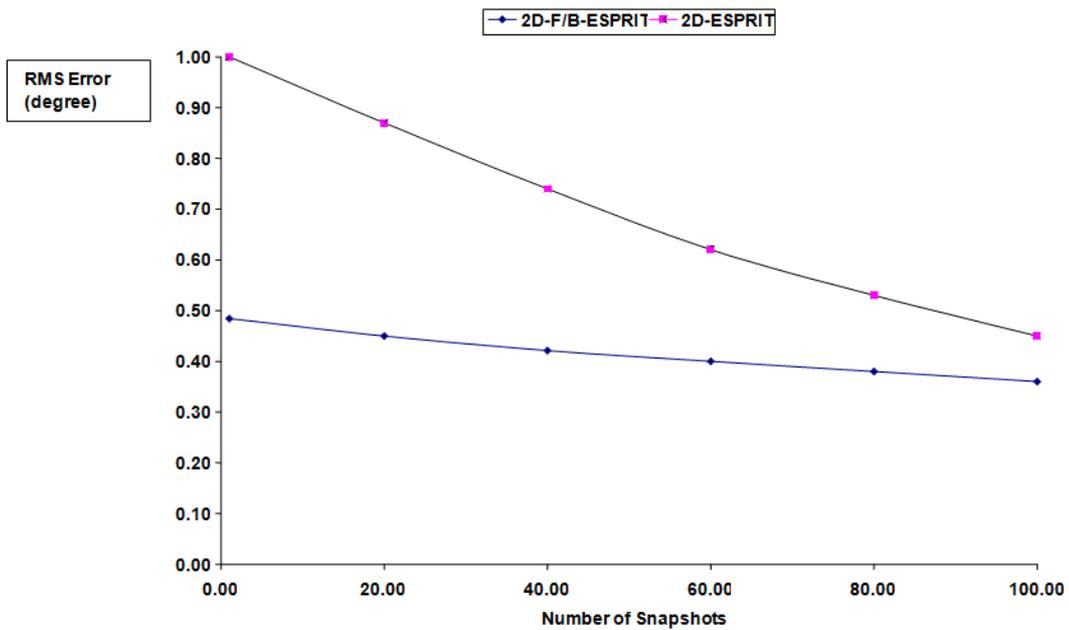
Figure -7: Root mean square error (RMS in degree) of the azimuth angle versus the number of snapshots
